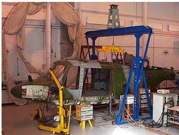
Figure 3 Test of Lynx Mk. 7 airframe at QinetiQ Farnborough
