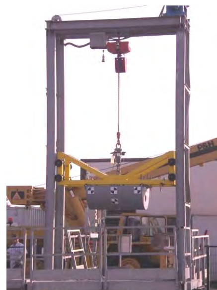
Figure 5 CIRA's LISA drop test facility
