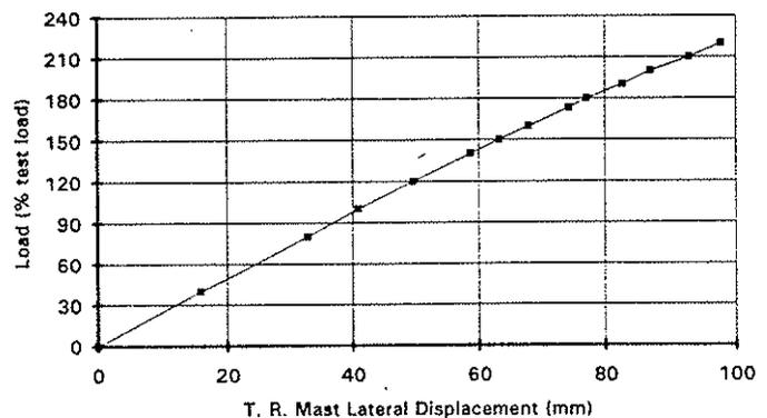
Fig. 11: Full scale static test load-displacement curve
