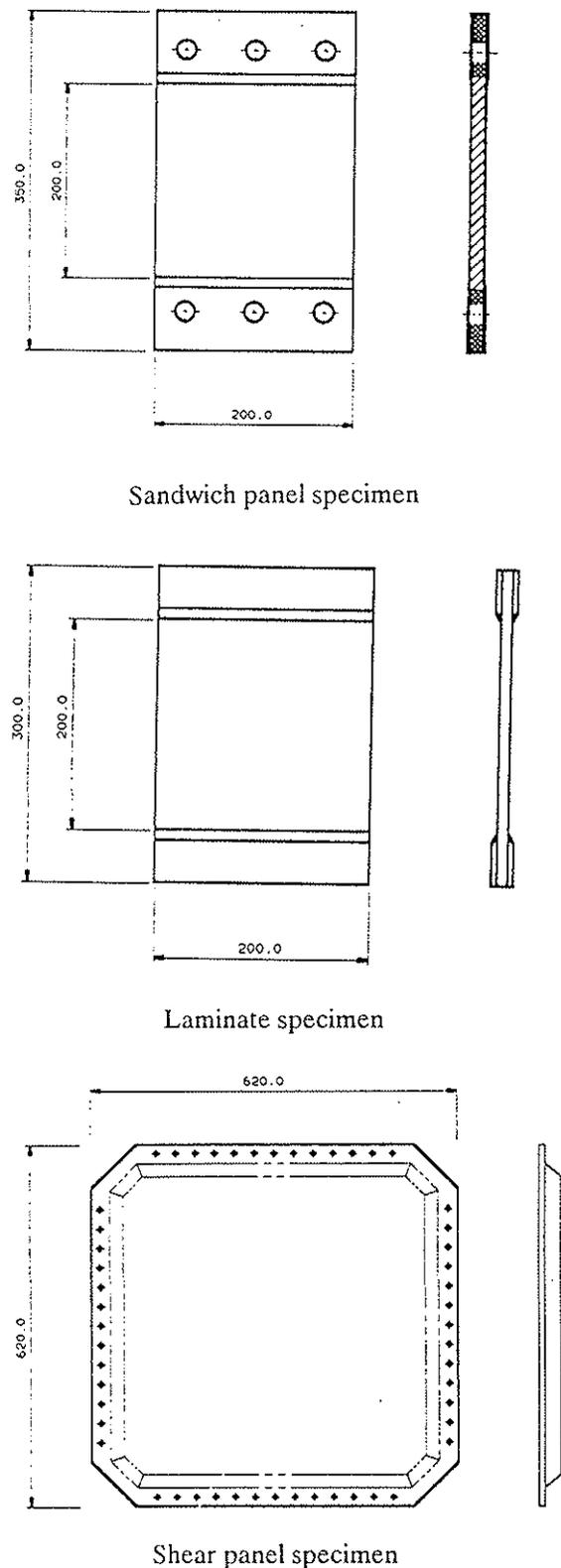
Fig.7: Specimens for material variability determination
