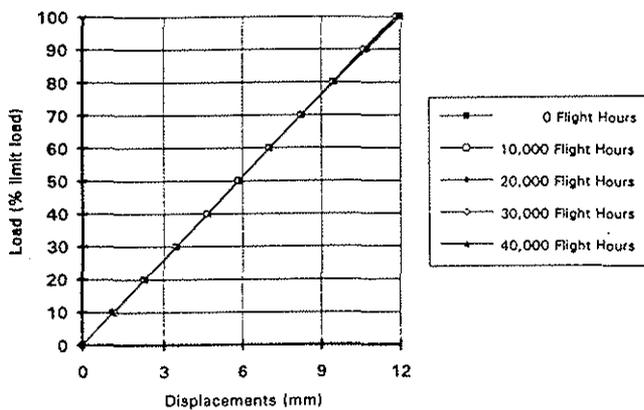
Fig.17: Fwd Spar Subcomponent stiffness variation
