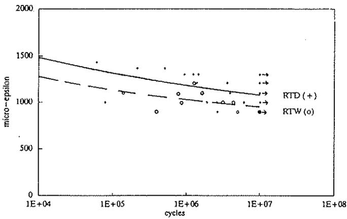
Fig.15: Humidity effect on sandwich panel S-N curve
