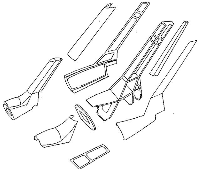
Fig.2: Tail Unit structure
