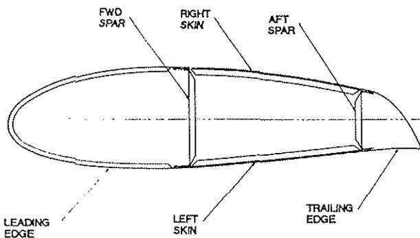
Fig.4: Vertical Fin cross section
