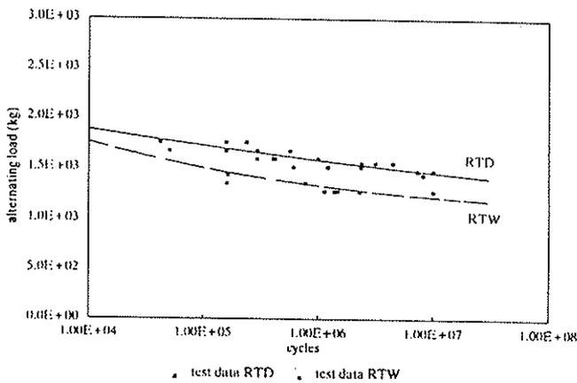
Fig.16: Humidity effect on joint
