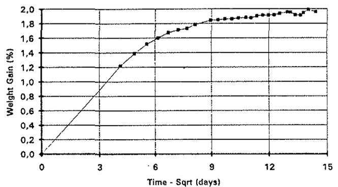
Fig.8: Sandwich panels moisture absorption curve
