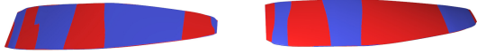
Figure 6: Upper (right) and lower (left) surfaces of the blade obtained with scanned points (blue) and interpolated laws (red).
