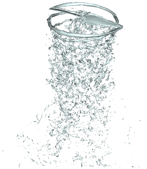
Figure 10: \lambda_2 criterion for RANS/LES.
