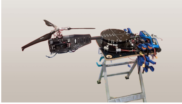
Figure 11. Setup of the balance used to perform the phase lag measurements on the T-H3 tiltrotor.
