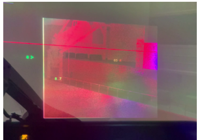
Figure 2. 3D conformal TRAGVIS sensor simulation image of a disabled container ship in the HMD (Secondary task)
