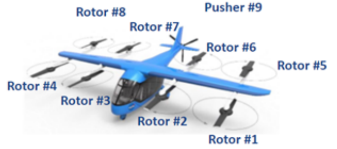
Figure 3: Lift-Plus-Cruise AAM Configuration from Ref. 10, 11
