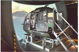
Fig. 12: Rotorcraft Simulation Environment (ROSIE)
