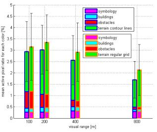
Fig. 9: Comparison of mean active pixel ratios; left bars: terrain with contour lines; right bars: terrain with regular grid
