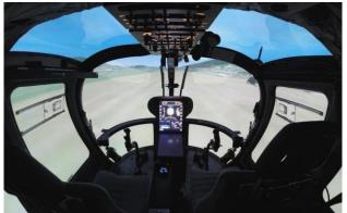
Fig. 14: Slim cockpit configuration of ROSIE with only two displays head down
