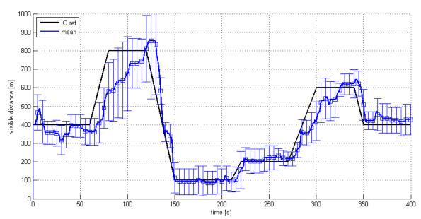
Fig. 15: Mean visible distance setting on the HMD according to the simulated Image Generator (IG) reference
