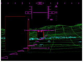
Fig. 8: A different scenery visualization variant: Terrain with regular grid and obstacles with bounding boxes
