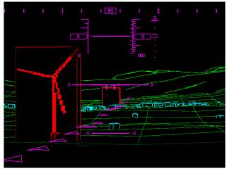
Fig. 10: Combination of terrain and obstacle visualization variants
