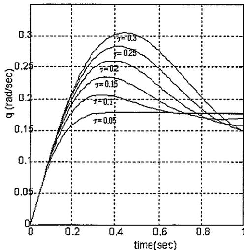
Fig. 3 Influence of  $da_1/dt$  on the pitch response of a semi-rigid rotor
