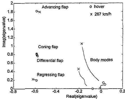
Fig. 6a Puma Body and Flap Eigenvalues as a Function of Forward Speed
