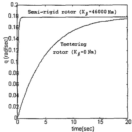
Fig. 2 Pitch response after a  $\theta_s$  step input for a semirigid and teeter configuration
