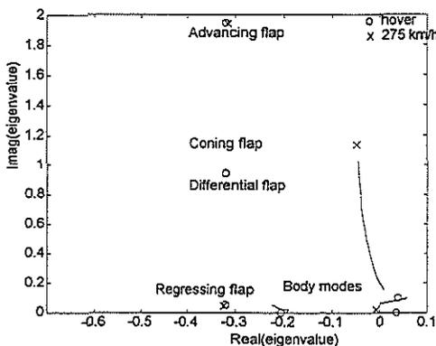
Fig. 6b Bo 105 Body and Flap Eigenvalues as a Function of Forward Speed
