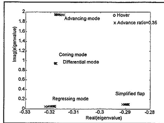
Fig. A-1b BO 105 Eigenvalues for the Complete and Simplified Flapping Equation
