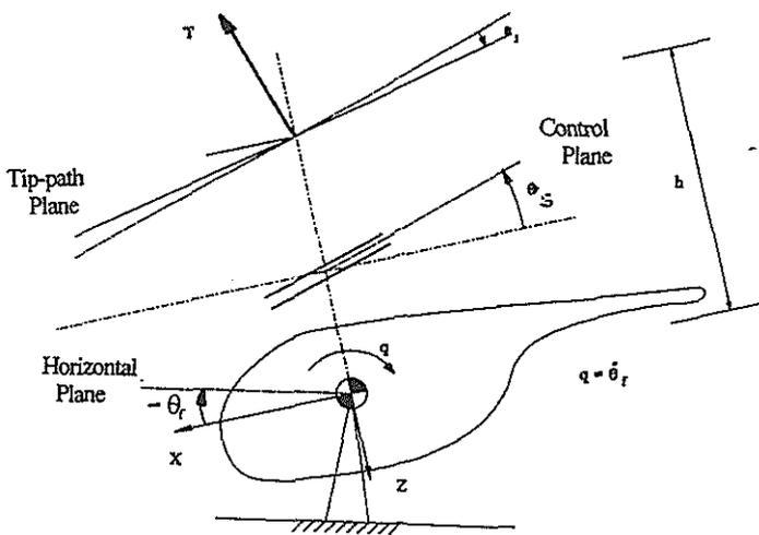
Fig. 1 Helicopter pitch motion after a longitudinal cyclic pitch step
