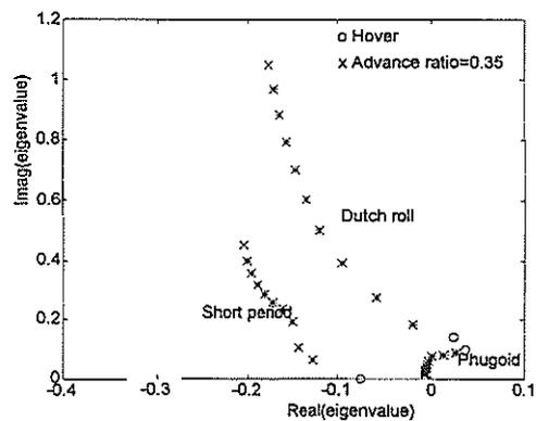
Fig. 5a Loci of Puma Eigenvalues with the Advance Ratio
