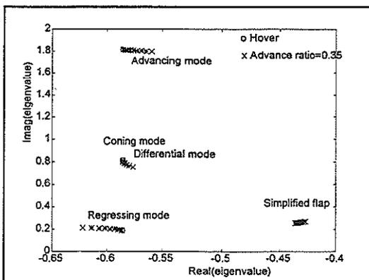
Fig. A-1a Puma Flap Eigenvalues for the Complete and Simplified Flapping Equation
