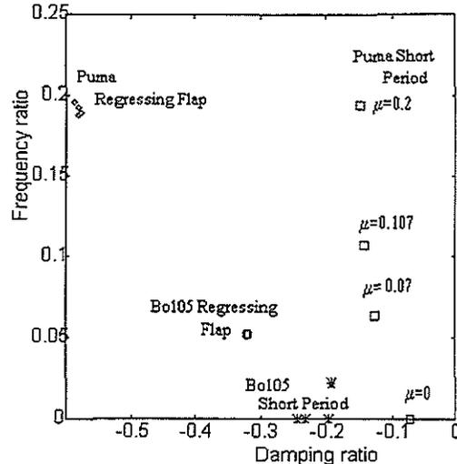
Fig. 7 Short period mode and flapping regressive mode for Puma and Bo105
