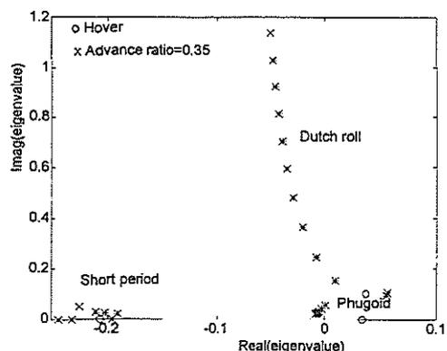
Fig. 5b Loci of Bo105 Eigenvalues with the Advance Ratio
