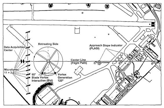
Figure 4: Arrangement of Test Equipment on Ground
