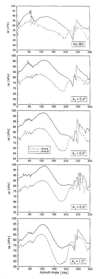
Figure 14: Leading edge blade pressure distribution for the 2/rev IBC amplitude sweep (6° approach, 65 KIAS). To check the wind tunnel observation of an increased noise reduction efficiency for multi-frequency inputs, a 3/rev+5/rev schedule was studied using 270° as fixed 3/rev phase angle and varying 5/rev phase angles.
