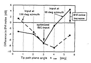
Figure 1: Noise Radiation versus Tip Path Plane Angle for two different IBC settings (from Ref. [2])
