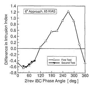
Figure 12: Reduction of intrusion index for varying 2/rev, 1° amplitude IBC phase angle (6° approach, 65 KIAS).
