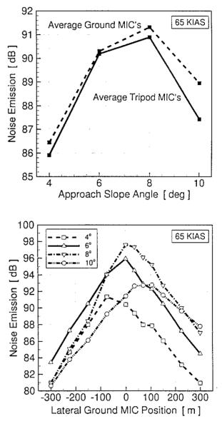
Figure 5: Noise emission for various approach slope angles at 65 KIAS, IBC not activated.
