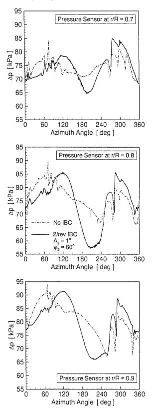
Figure 11: Leading edge blade pressure distribution versus azimuth angle for three radial stations (6° approach, 65 KIAS).
