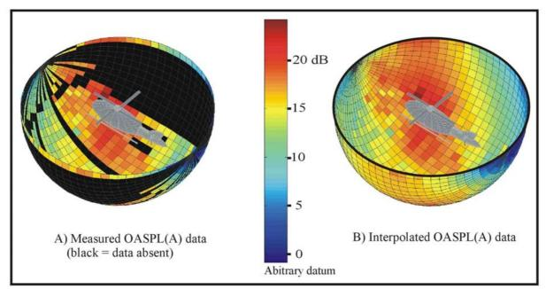
*Figure 15. Directivity hemisphere for OASPL (A), from data measured from flight at 35m and 200m, and interpolation to fill in the gaps. Constructed from 1/3<sup>rd</sup> Octave directivity. Flight speed is 90 kts.*
