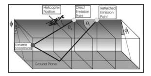
Figure 8. Incident and reflected rays for a highly elevated microphone.
