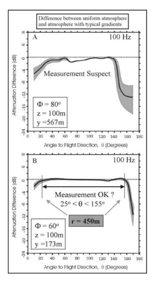
Figure 6. Influence of refraction, as a function of  $\theta$ , on measurements for  $\phi = 60^{\circ}$ ,  $80^{\circ}$  for a fly-by at 100m above ground level.
