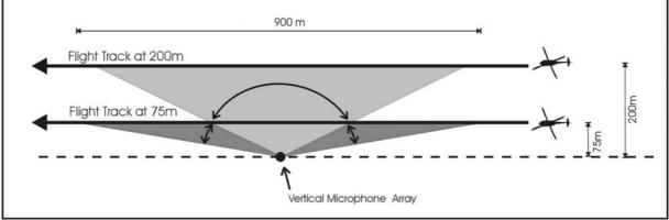
Figure 9. Ranges of  $\theta$  covered by vertical arrays at 75m and 200m.
