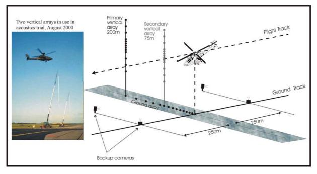
Figure 12. Arrangement of microphones used in HAMSTER for helicopter acoustic characterisation
