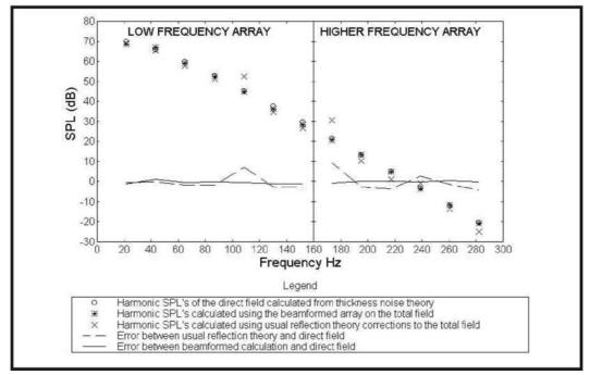
Figure 11. Beamform performance compared with standard reflection corrections using theoretical data.
