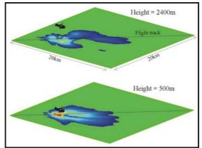
Figure16. Effect of different flight heights on OASPL(A) noise contours for level flight at 90 kts.
