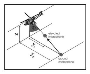
Figure 7. Elevation of microphone to reduce radiation distance.ground,
