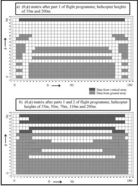
Figure 13. Matrix of angles  $(\theta, \phi)$  covered, in bins of 5°, by a range of flight heights.
