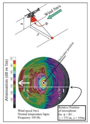
Figure 5. Effects of atmospheric refraction, calculated using MAPE [4].
