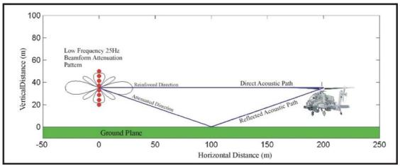
Figure 10. Beamform attenuation pattern for array A at 25 Hz
