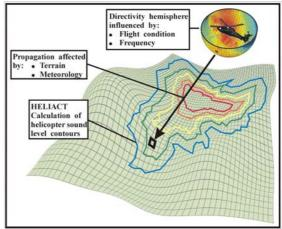
Figure 2. HELIACT - Helicopter Acoustic Contouring Tool
