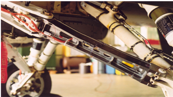
Figure 10: TiMMC LDB installed on F-16
