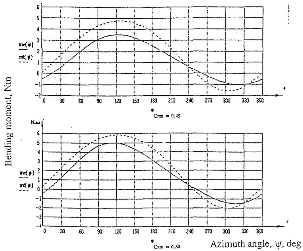
Fig. 3 Comparison of analytical and experimental flatwise bending moment results
