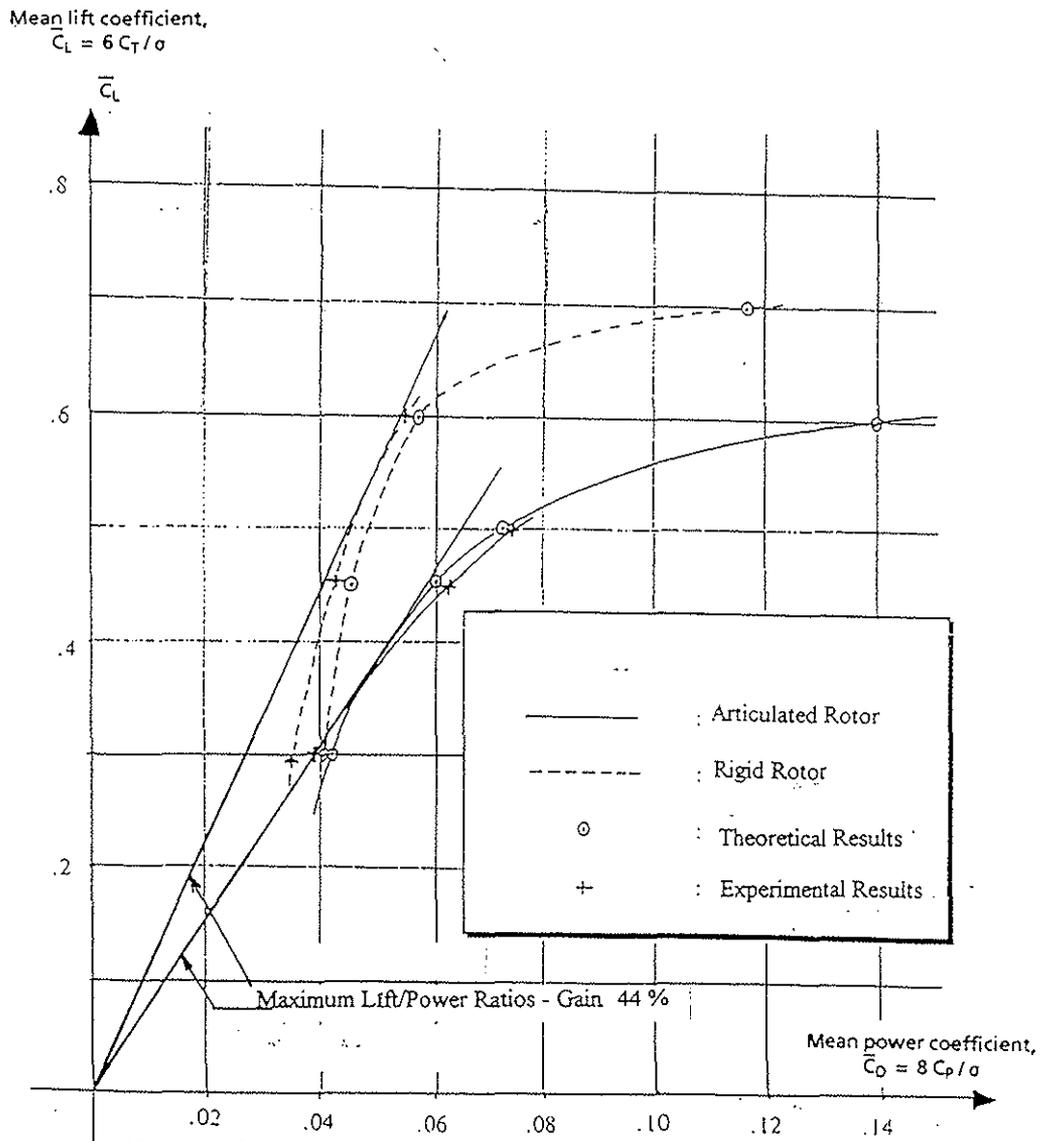
Fig. 4 : Comparison of rigid and conventional rotor performance
