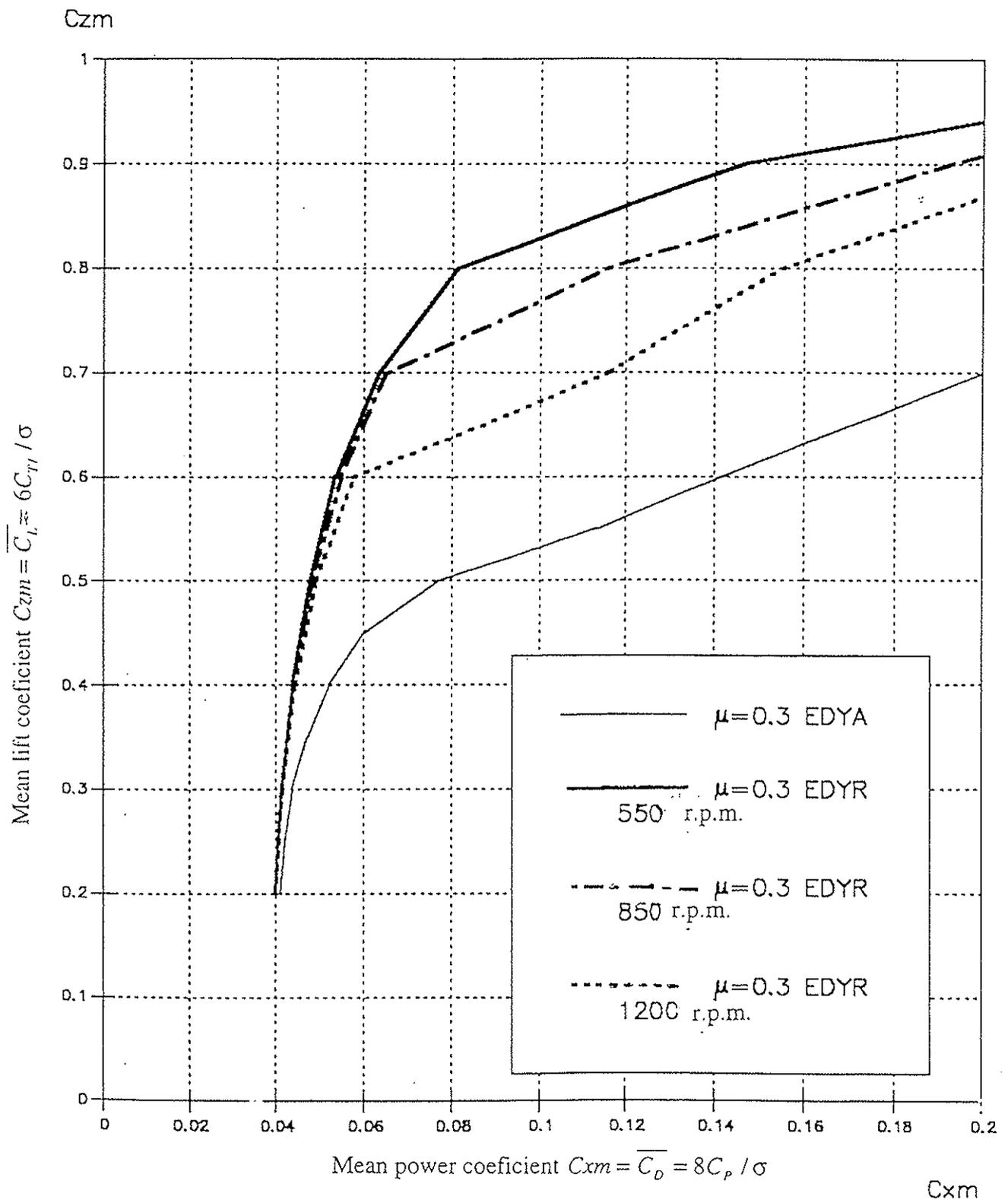
Fig. 7 : Theoretical polar diagrams of EDY R and EDY A rotors at  $\mu = 0.3$ ,  $\overline{S_f} = 0.1$
