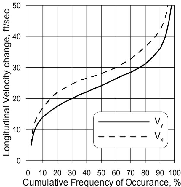
Fig. 1 Change of speed for survivable accidents of rotary-wing and light aircrafts with a fixed wing.
