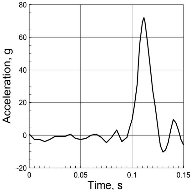
Fig. 6. Overloads on a cargo compartment floor location.
