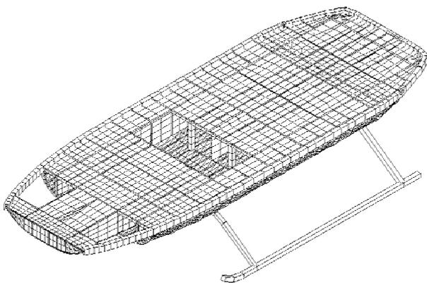
Fig. 3 General view of finite-element model of lower panel.
