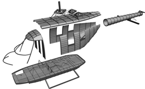
Fig. 2 Complete finite-element model of the helicopter for calculation of static strength and modal characteristics.
