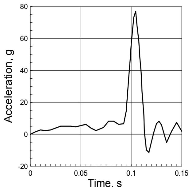
Fig. 5. Overloads on a pilot seat floor location.
