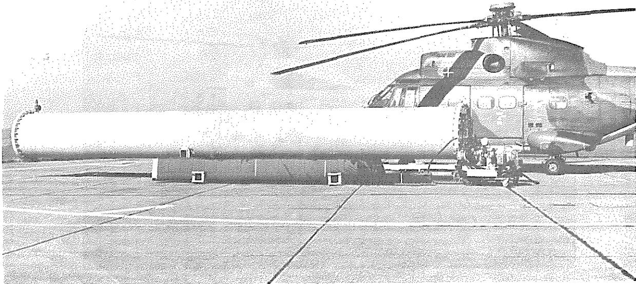
Fig 5 Test chamber for pressure sensor calibration
