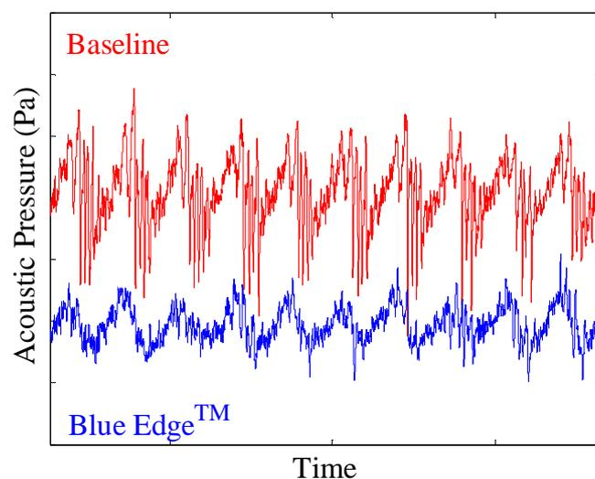
**Figure 17 : Acoustic pressure time-history at 2 (60m before overhead position) for reference and Blue Edge<sup>TM</sup> blades for a 60 kt,  $-8^\circ$  glideslope approach.**
