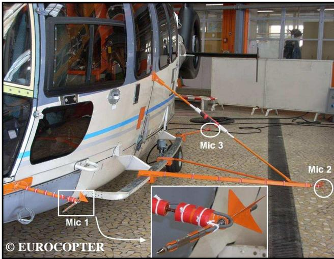
**Figure 4 : Near-field microphone installation.**
