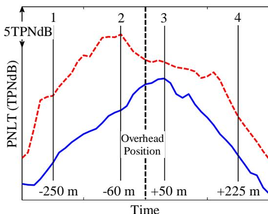
**Figure 12 : Tone-Corrected Perceive Noise Level time-history for reference (red dashed curve) and Blue Edge™ (blue solid curve) rotors for a 60 kt,  $-8^\circ$  glideslope approach.**
