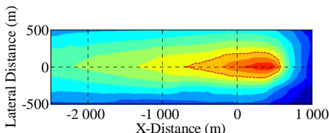
**Figure 21 : EPNL noise footprint prediction for Blue Edge™ rotor in approach phase at 60kt, -8° glideslope (colour contours are 2 EPNdB apart).**
