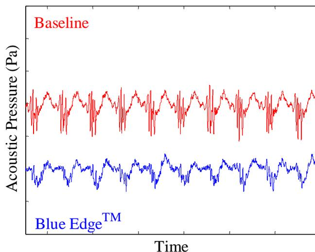
**Figure 13 : Acoustic pressure time-history at point 1 (see Figure 12) for reference and Blue Edge™ blades for a 60 kt,  $-8^\circ$  glideslope approach (pressure scales are identical).**
