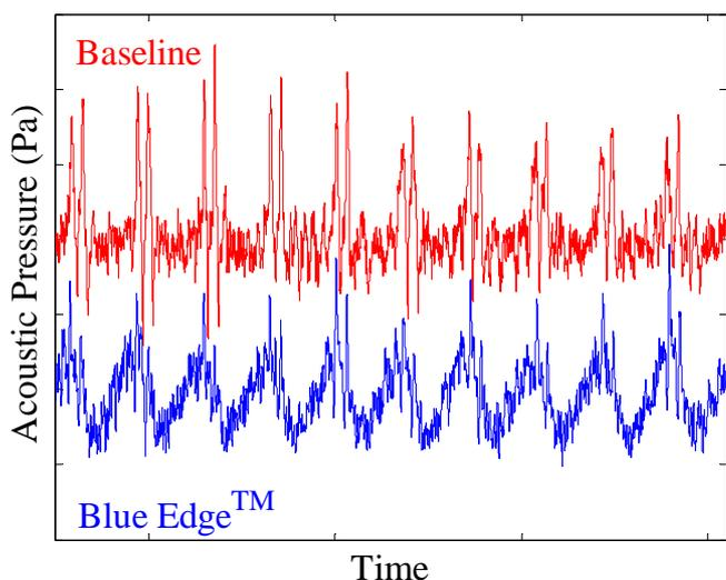
**Figure 18 : Acoustic pressure time-history at 3 (50m after overhead position) for reference and Blue Edge™ blades for a 60 kt, -8° glideslope approach.**
