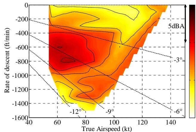
**Figure 5 : Near-field A-weighted sound pressure level for reference rotor (contours are 2dB(A) apart).**
