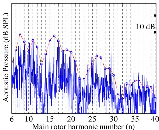
**Figure 15 : Sound Pressure level as a function of Blue Edge<sup>TM</sup> rotor harmonic at point 1 (Figure 13) for a 60 kt,  $-8^\circ$  glideslope approach.**
