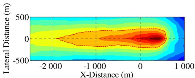
**Figure 20 : EPNL noise footprint prediction for baseline rotor in approach phase at 60kt, -8° glideslope (colour contours are 2 EPNdB apart).**
