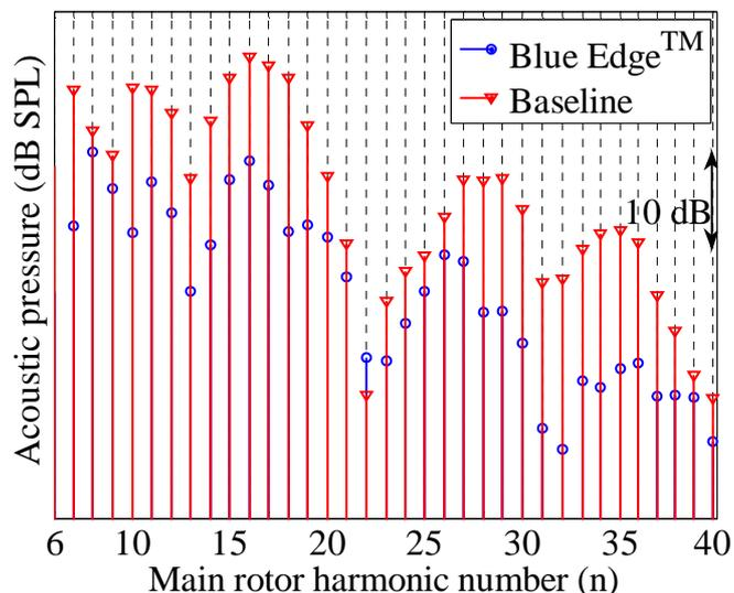
**Figure 16 : Sound Pressure level for 6<sup>th</sup> to 40<sup>th</sup> rotor harmonics for baseline and Blue Edge rotors at point 1 (Figure 13) for a 60 kt,  $-8^\circ$  glideslope approach.**
