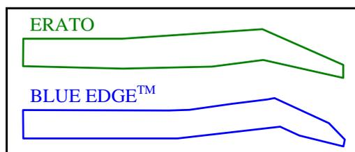
Figure 2 : Comparison of the blade planform between ERATO and Blue Edge™
