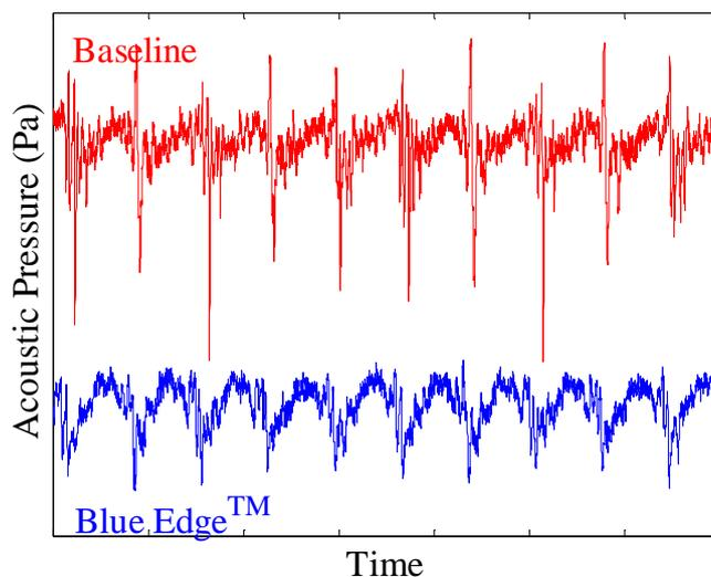
**Figure 8 : Acoustic pressure time-history for standard and Blue Edge™ blades for a 55 kt, -4° glideslope approach (pressure scales are identical).**
