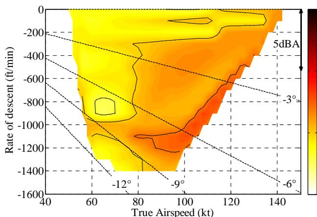
**Figure 6 : Near-field A-weighted sound pressure level for Blue Edge™ rotor (contours are 2dBA apart).**
