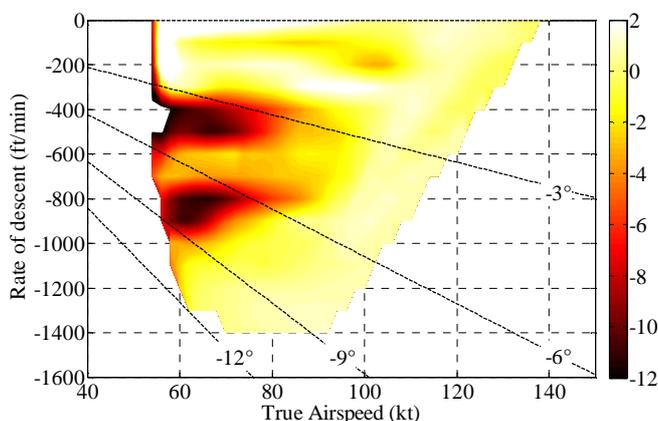
**Figure 7 : Difference between near-field kurtosis for the two rotors (negative values where reference rotor has higher kurtosis).**
