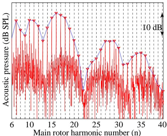
**Figure 14 : Sound Pressure level as a function of baseline rotor harmonics at point 1 (Figure 12) for a 60 kt,  $-8^\circ$  glideslope approach.**
