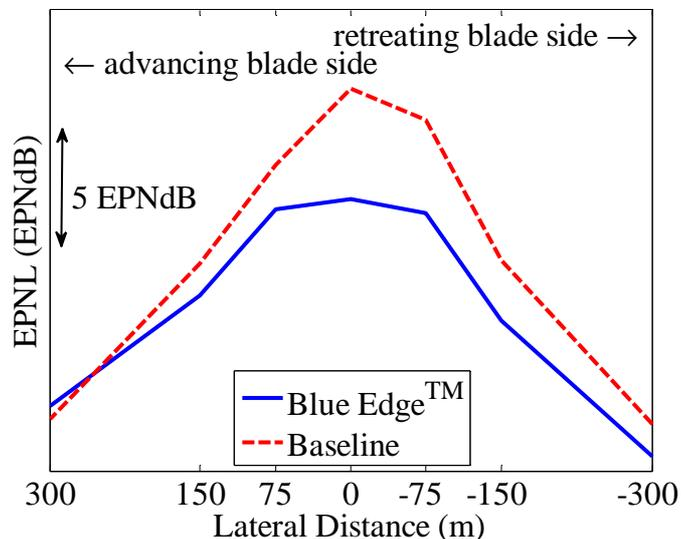
**Figure 9 : EPNL as a function of lateral distance for baseline and Blue Edge™ rotors.**
