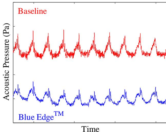
**Figure 19 : Acoustic pressure time-history at point 4 (225m after overhead position) for reference and Blue Edge™ blades for a 60 kt, -8° glideslope approach.**
