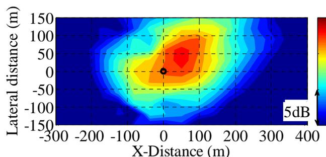
**Figure 11 : Noise footprint for isolated Blue Edge™ rotor computed with HMMAP prediction tool.**
