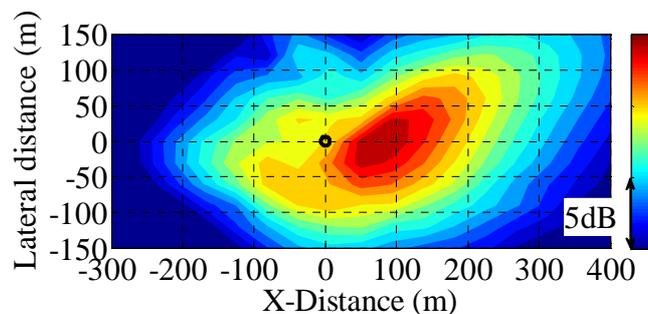
**Figure 10 : Noise footprint for isolated reference rotor computed with HMMAP prediction tool.**
