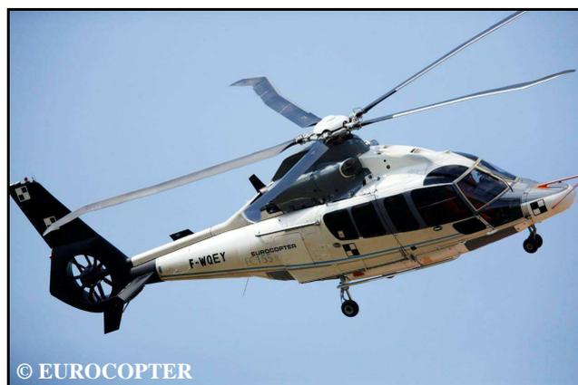
Figure 3 : EC155 equipped with Blue Edge™ blades during noise measurements.
