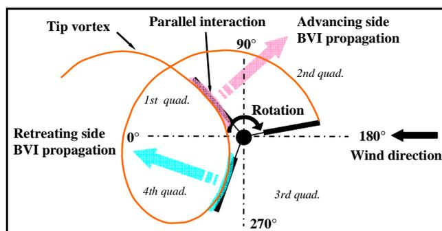
**Figure 1 : Typical parallel Blade-Vortex Interactions on the advancing and retreating blade sides**
