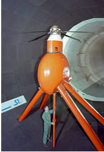
Figure 1: ERATO setup in ONERA’s S1MA wind tunnel.
