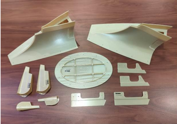
Fig. 28: Secondary tail parts manufactured by thermoplastic additive layer techniques.
