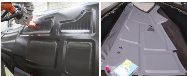
Fig. 5: Robotic automated fiber placement of the starboard side shell (by courtesy of Fraunhofer IGCV); primed and trimmed side shell ready for installation.
