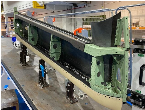
Fig. 22: Build of the lower wing fully drilled and fastened ready for integration with upper wing and cradle.
