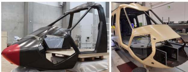
Fig. 9: Canopy and nose structure with hybrid radome; installed canopy (courtesy KLK).
