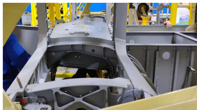
Fig. 7: Main landing gear section (stub wing and center fuselage) with frame 4 and 5, root and end ribs, stringer-stiffened longerons, sandwich center keel beam, machined structural floor (by courtesy of the Romanian consortium RoRcraft).
