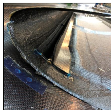
Fig. 18: Structurally bonded upper spar boom T-return to upper cover at D-nose perimeter.
