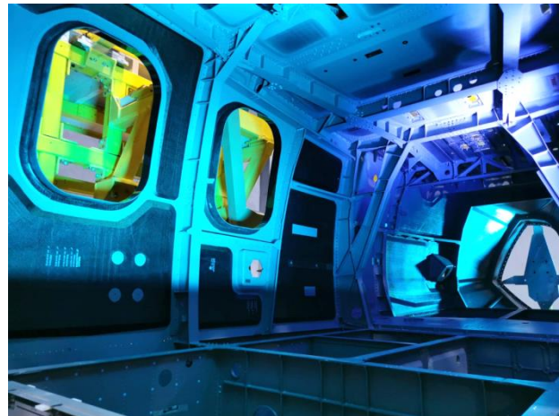
Fig. 6: Inner view of the fuselage assembly: subfloor structure, side shells and machined metallic framework members (by courtesy of the Romanian consortium RoRcraft).
