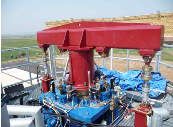
Figure 4 3-axis load balance Calibration of WTTF
