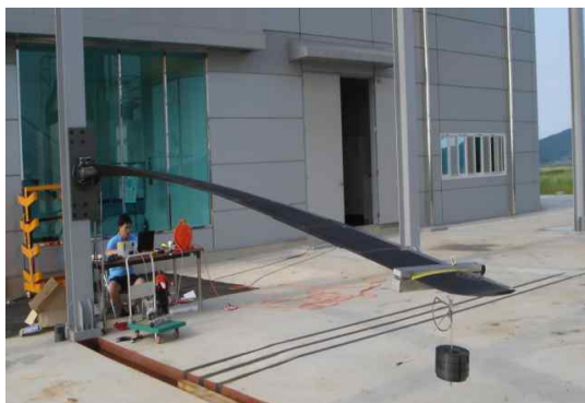
Figure 10 Load Calibration of Main Rotor Blade
