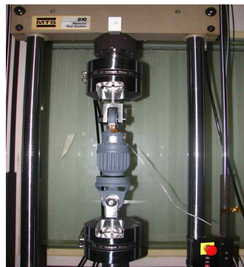
Figure 7 Damper Calibration for Rotor Hub System
