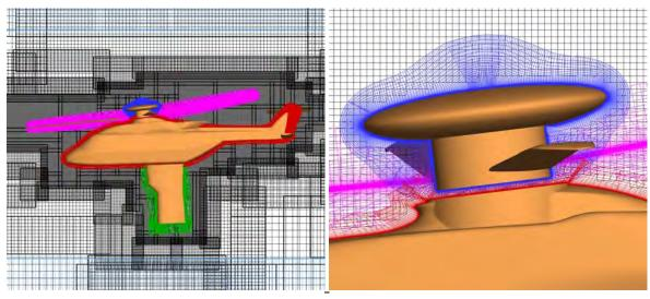
Figure 1 - Close-up view of the global mesh (left) and of the Chimera blanking near the hub (right)
