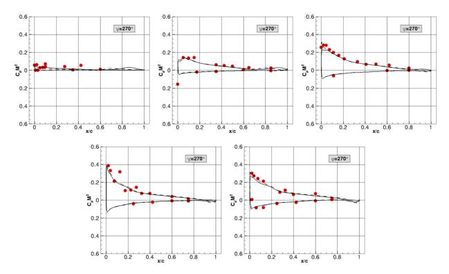
Figure 10 - Sectional surface pressure data (CpM2) for the main rotor at retreating side for the cruise and highspeed tail-shake test case. Solutions are shown at r/R=0.5 - 0.7 - 0.825 - 0.915 - 0.975 section position on the blade (dashed line = blind test, solid line = post test)
