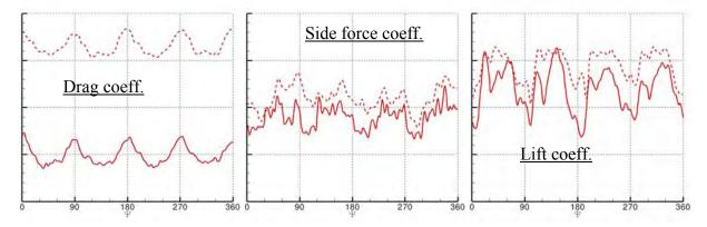
Figure 5 - Force data of the helicopter fuselage for the cruise and high-speed tail-shake test case (dashed line = blind test, solid line = post test)
