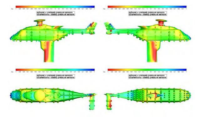
Figure 7 - Surface pressure coefficient Cp for the cruise and high-speed tail-shake test case at main rotor azimuth  $\psi$ =60°
