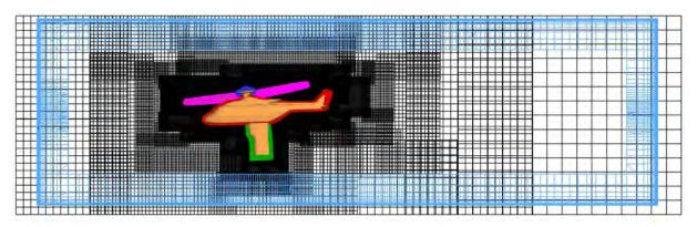
Figure 2 - Cartesian off-body grids extension out of the wind tunnel walls
