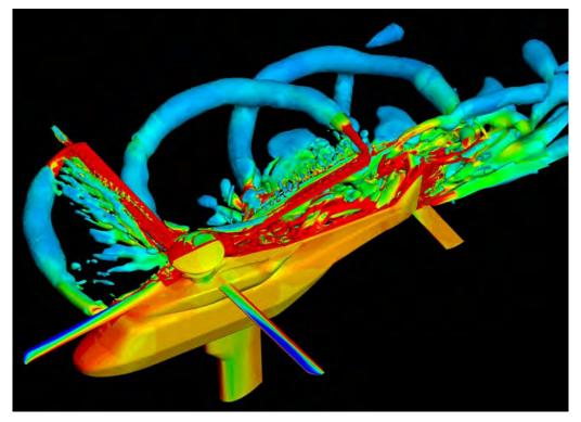
Figure 4 - Colored view of the flow solution around the GOAHEAD configuration (pressure coefficient on wall surfaces and wakes represented by isosurface of Q criteria)
