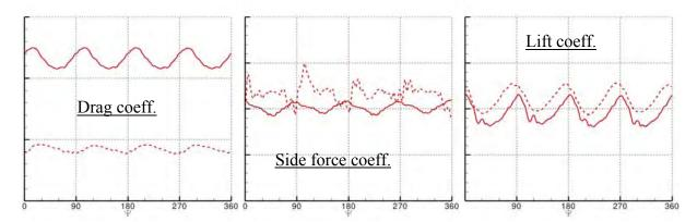
Figure 6 - Force data of the main rotor for the cruise and high-speed tail-shake test case (dashed line = blind test, solid line = post test)
