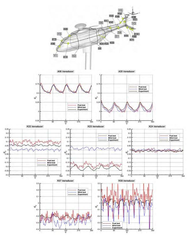
Figure 8 - Location and results of pressure sensor data (Cp) for the cruise and high-speed tail-shake test case (black line = experiment, blue line = blind test, red line = post test)
