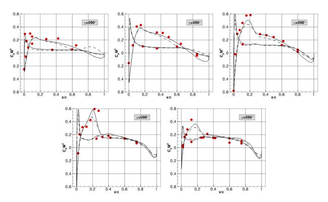
Figure 9 - Sectional surface pressure data (CpM2) for the main rotor at advancing side for the cruise and highspeed tail-shake test case. Solutions are shown at r/R=0.5 - 0.7 - 0.825 - 0.915 - 0.975 section position on the blade (dashed line = blind test, solid line = post test)
