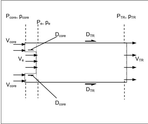
Figure 2 Control Volume for the Core Section
