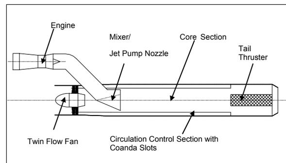
Figure 1 Schematic of the CIRSTEL Tail Boom
