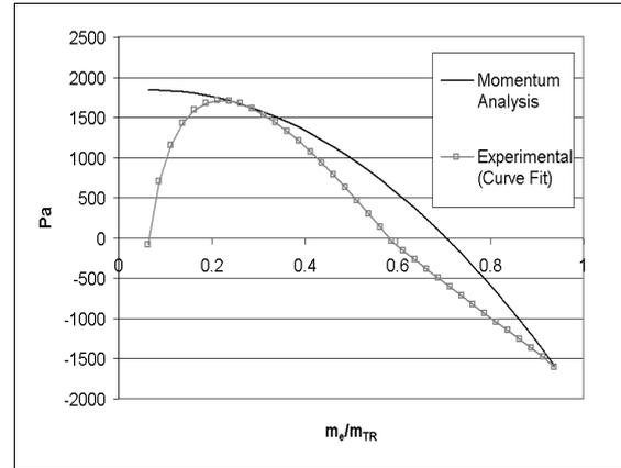
Figure 3 Momentum Analysis and Experimental Result Comparison for the Core Section
