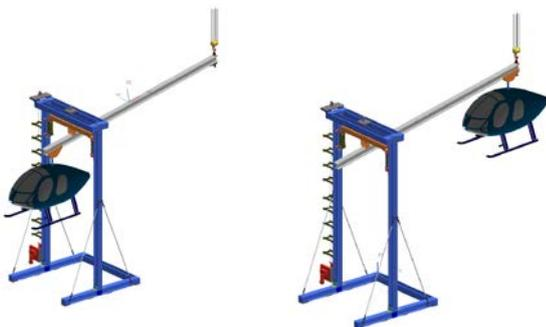
Figure 11. Full-Scale Aircraft Drop Test Set-Up
