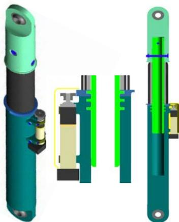
Figure 4. Prototype LLSE to limit the Major Mass Item loads during a crash impact.
