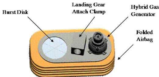
Figure 10. External Airbag Assembly including the Burst Disk and Hybrid Gas Generator
