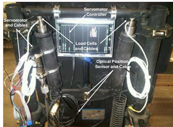
Figure 3. ASEA installation on a Rotorcraft Crew Seat
