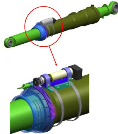
Figure 8. Shock Strut Active Load Control Implementation
