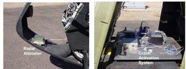
Figure 12. ACPS Hardware and Radar Altimeter installation for the Drop Test Aircraft
