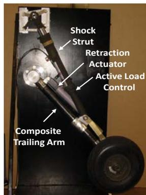
Figure 7. Prototype Smart Crashworthy Landing Gear
