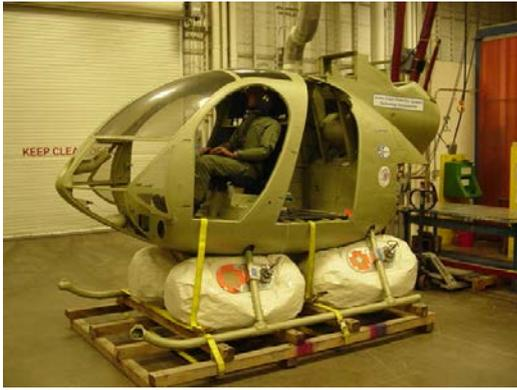
Figure 9. Prototype External Airbag System
