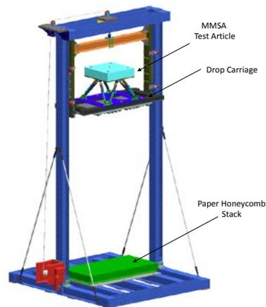
Figure 5. Major Mass Structural Assembly (MMSA) Drop Test Setup
