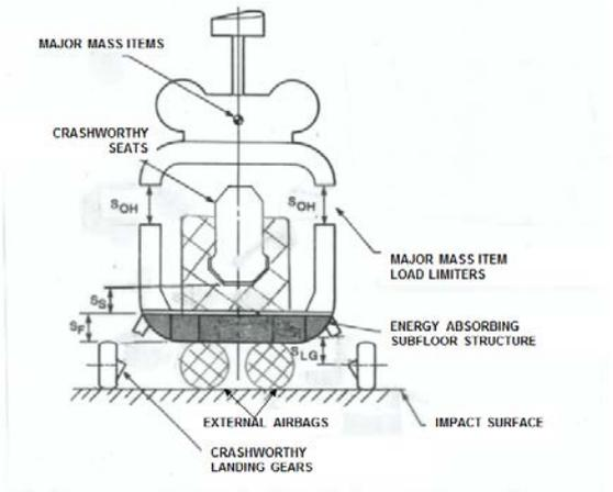
Figure 1. Crashworthy Subsystems and Energy Absorbing Airframe Structures
