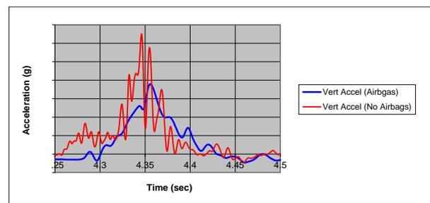
Figure 13. Full-Scale Aircraft Drop Test Vertical Accelerations
