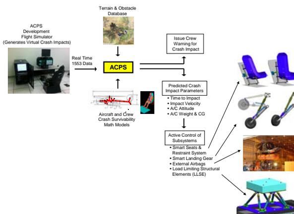
Figure 14. ACPS Architecture shown in a Hardware-in-the-Loop Simulation Configuration.
