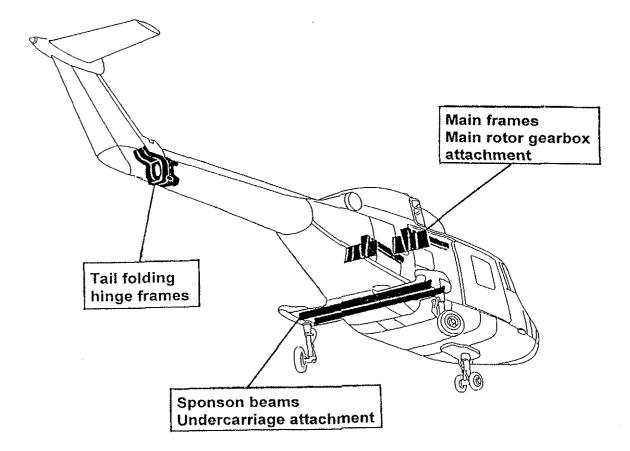
Figure 1: Fatigue sensitive and life limited area of Lynx airframe.
