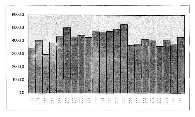
Figure 2: Distribution of consumed life over fleet: flying hours vs.aircraft registration number.
