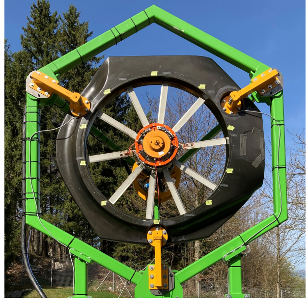
Figure 1: Rear view of the tail rotor test rig.
