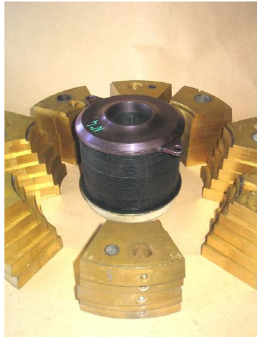
Figure 18: CF bearing mould components. PAULSTRA photo
