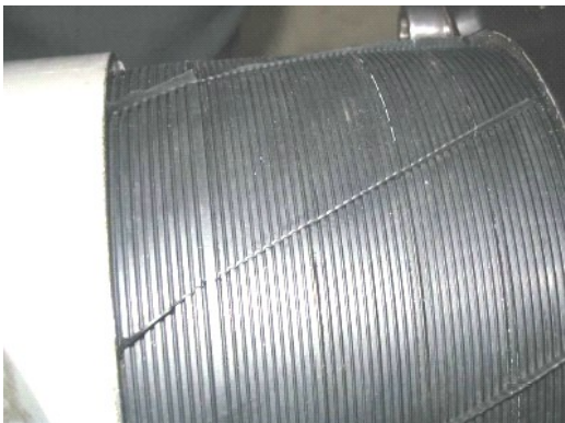
Figure 33: 44° Torsion of CF bearing. PAULSTRA photo
