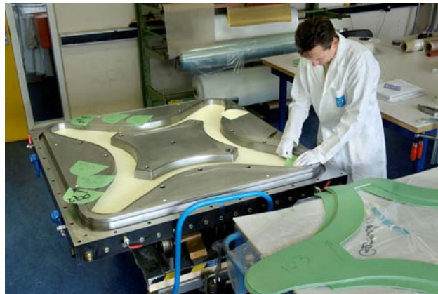
Figure 10 : Yoke lower mould during laminating. NLR photo
