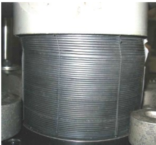
Figure 34: 3° cocking on CF bearing. PAULSTRA photo
