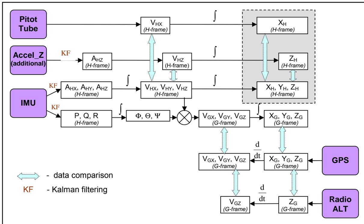
Fig. 5 The flow diagram of signal acquisition and processing
