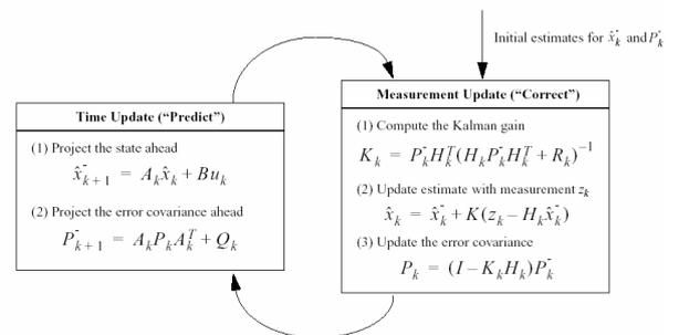
**Fig. 4** The flow chart of the discrete Kalman filtering process.
