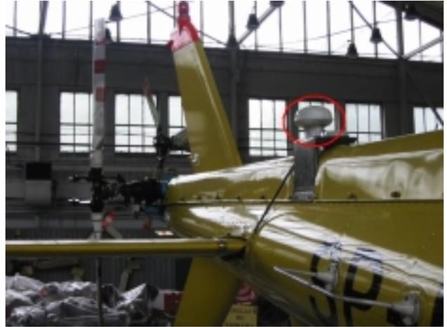
**Fig. 3** Point of placement of the SmartAntenna.
