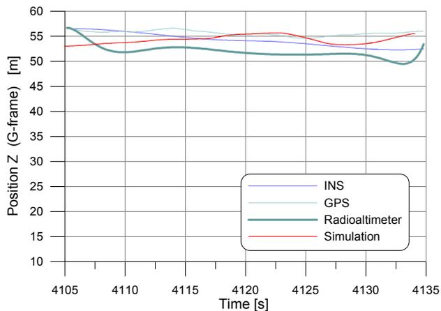
**Fig. 9** Altitude of the helicopter's level flight
