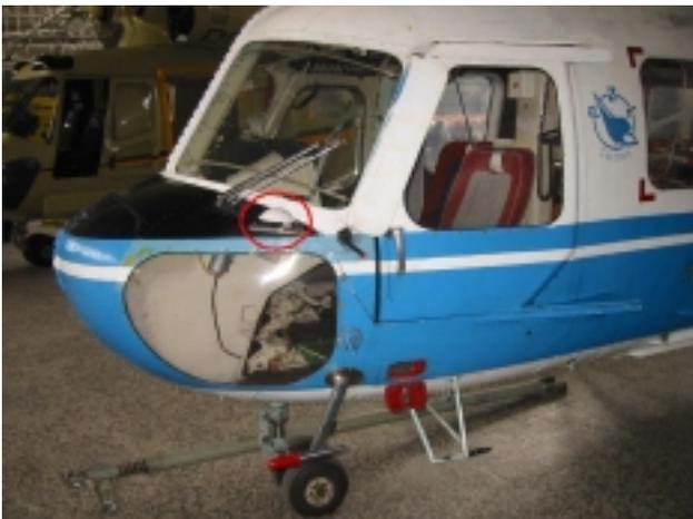
**Fig. 2** Point of the placement of the ProPak II Millennium receiver's antenna.
