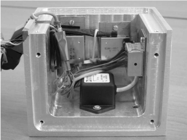
**Fig. 1** The Inertial Navigation Unit developed in Warsaw University of Technology
