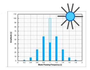
Figure 4: Simulated spectrum of a modulated Fenestron™ rotor from [6].
