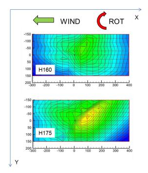
Figure 15: HMMAP simulated noise footprints for H160-B (above) and H175-B (below), 1 dB(A) / contour line.
