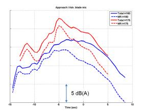
Figure 11: Total and main rotor tonal A-weighted noise level along observer time on H160-B and H175-B on advancing-side microphone.
