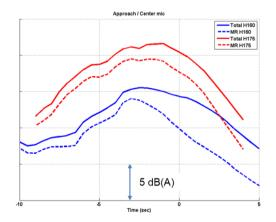
Figure 12: Total and main rotor tonal A-weighted noise level along observer time on H160-B and H175-B on center microphone.
