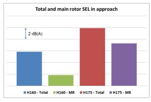
Figure 14: Total and ROSI-extracted main rotor SEL values on H160-B and H175-B.
