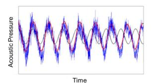
Figure 9: Example of extraction of reception BPF using ROSI.
