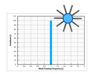
Figure 3: Simulated spectrum of a non-modulated Fenestron™ rotor from [6].
