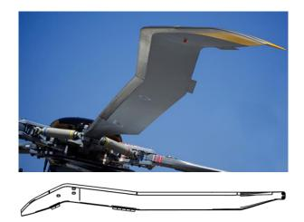
Figure 2: Blue Edge™ planform of H160-B main rotor.
