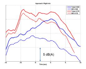
Figure 13: Total and main rotor tonal A-weighted noise level along observer time on H160-B and H175-B on retreating side microphone.
