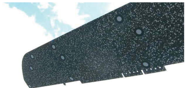
Figure 8: Rotor blade with speckle pattern and markers.
