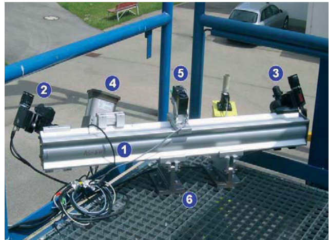
Figure 10: Camera system on the whirl tower ( 1 - support; 2,3 - cameras; 4 - strobe light; 5 - laser sensor; 6 - whirl tower platform).
