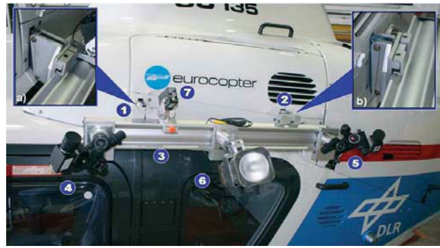
Figure 7: The experimental set-up installed at the helicopter (1, 2 – mountings; 3 – support; 4, 5 – cameras; 6 – strobe light; 7 – laser sensor ).
