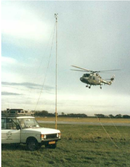
Figure 7 Shore based hover trials with the Lynx helicopter in 1981
