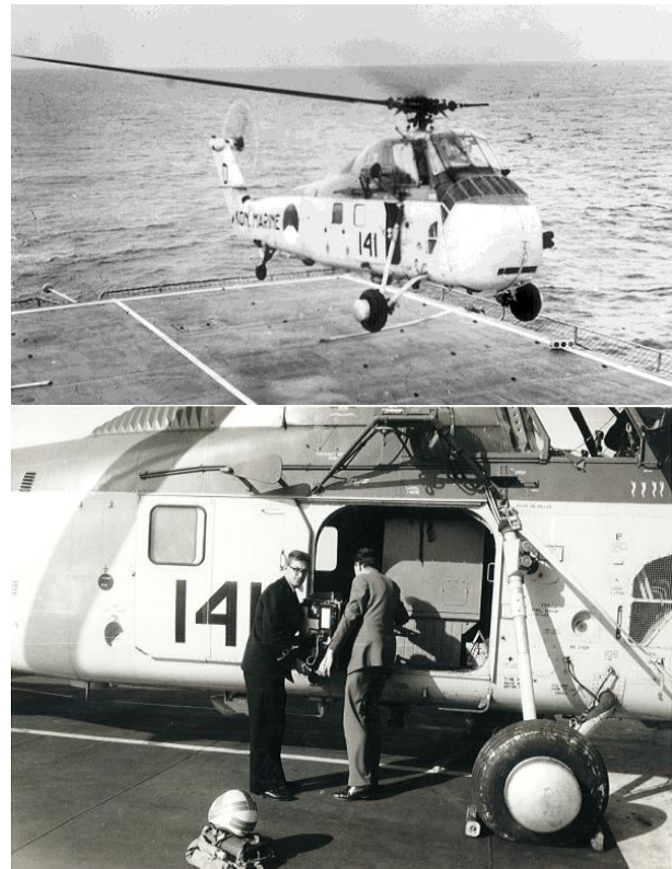
Figure 3 First Dutch helicopter-ship qualification trial with Sikorsky S-58 on board "Hr. Ms. Poolster".
