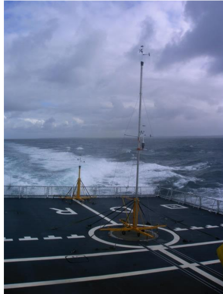
Figure 6 10m high measuring mast equipped with 3D anemometers to measure air flow at the helicopter deck. A second 3m high mast was added later.
