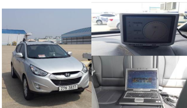
Figure 14 Pace car (left picture), display for pace car driver (right top picture) and data processing and recording system based on a laptop computer (right lower picture).
