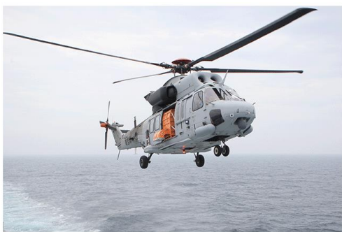
Figure 16 The KUH-1M at sea with the water tank installed (source: KAI)
