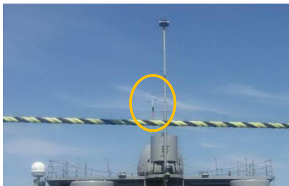
Figure 19: Reference anemometer at the jackstaff on the bow of ROKN LST
