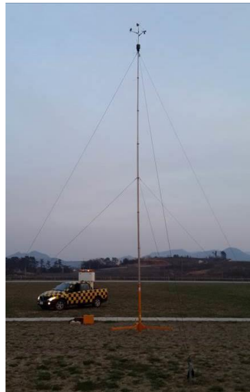
Figure 15: Mast with anemometer at Sacheon Airport
