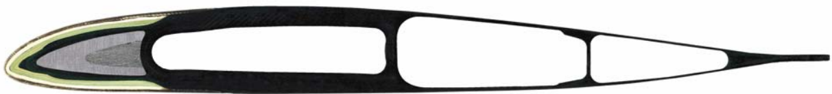
Typical main rotor blade 226 section ( blade chord B = 260 \text{ mm} )
