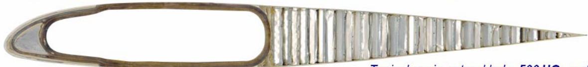
Typical main rotor blade 500 UG section ( blade chord B = 480 mm )
