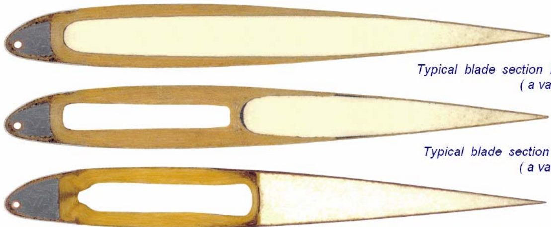
Typical production main rotor blade B - 7 section ( blade chord B = 260 \dots 104 mm, B_7 = 170 mm )
