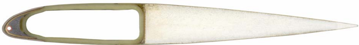
Typical main rotor blade N - 1M section ( blade chord B = 350 \dots 175 mm, B_7 = 250 mm )
