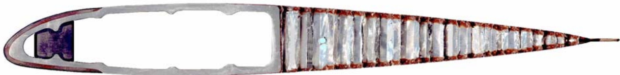
Typical main rotor blade D 1 - M section ( blade chord B = 370 mm )
