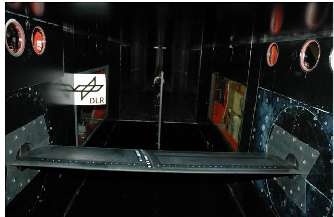
Figure 1: The OA209-FCD model installed in the adaptive-wall test section of the DNW-TWG.
