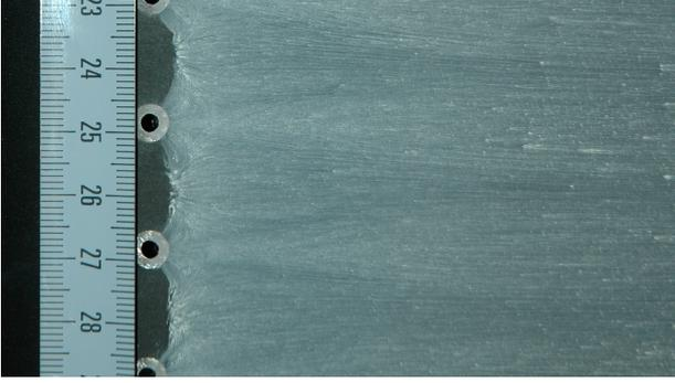
Figure 6: Oil flow picture for  $M=0.3$ ,  $Re=1.15e6$ ,  $\alpha=13^\circ$ ,  $P_j=10$  bar. Flow is from left to right.
