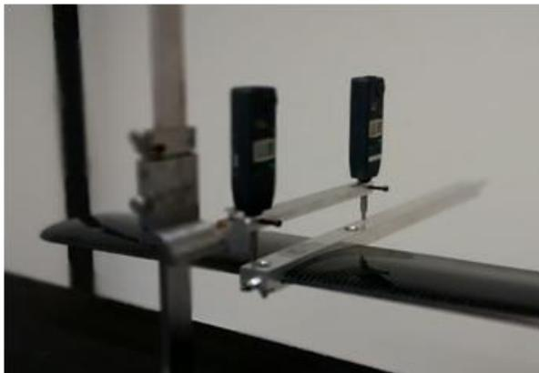
Figure 6 Stiffness testing setup
