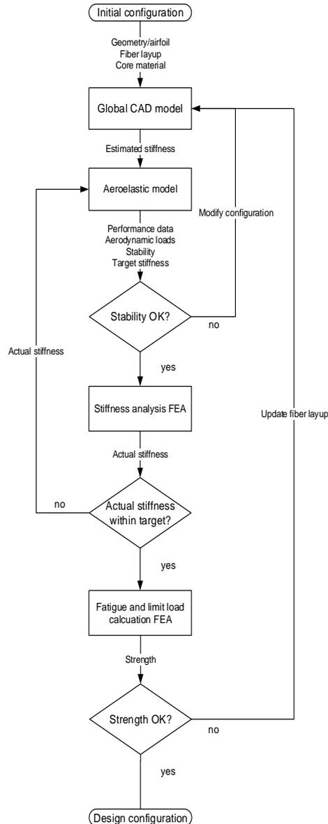
*Figure 2* Rotor blade design process
