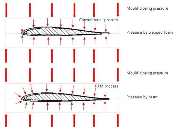
Figure 5 Pressure differences between conventional process and RTM process
