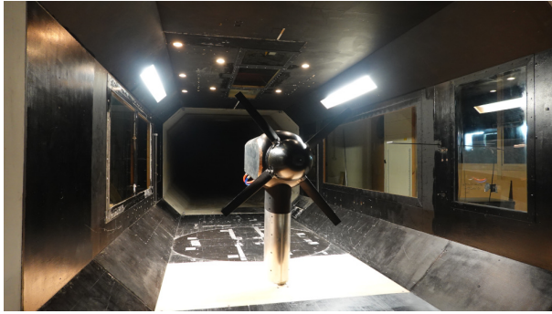
Figure 5: The UKNRR installed in the deHavilland tunnel.
