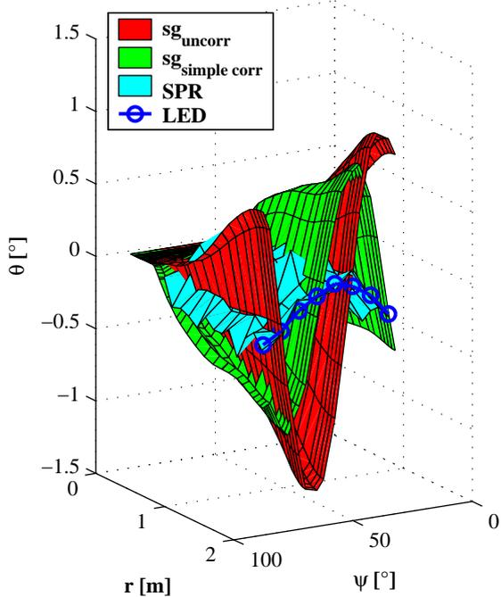
Figure 9: 6/rev twist deformation, all actuators active
