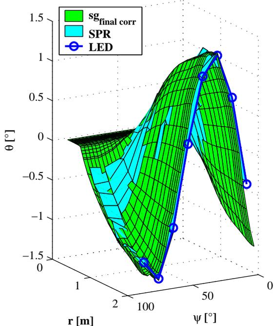
Figure 10: 4/rev deformation with final correction, all actuators active
