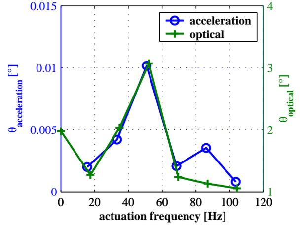
Figure 3: comparison optical and acceleration measurement of blade tip twist
