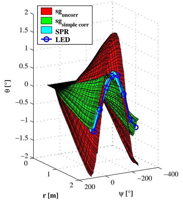
Figure 7:  $1/rev$  twist deformation, all actuators active
