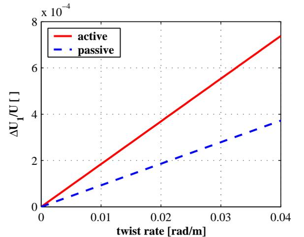
Figure 4: output of torsion bridge 1 as a function of twist rate
