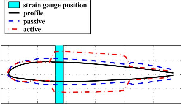
Figure 5: active and passive distribution of  $+45^\circ$  strain
