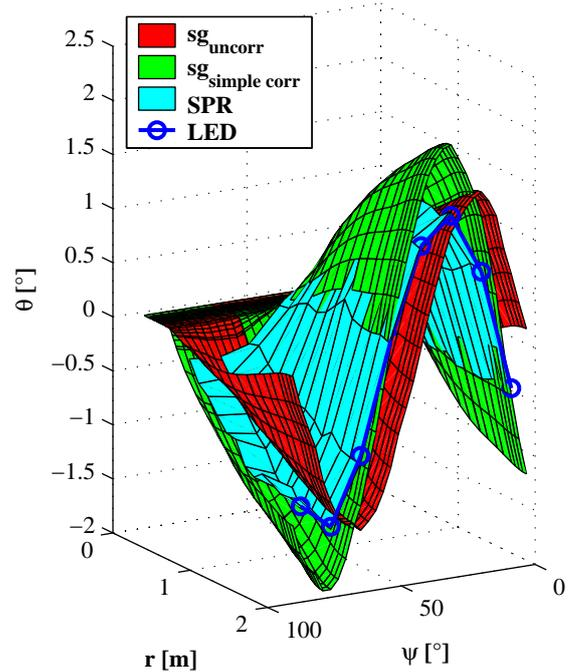
Figure 8:  $4/rev$  twist deformation, all actuators active
