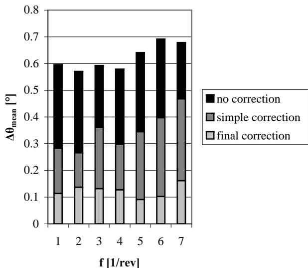
Figure 11: mean twist deviation as a function of actuation frequency, all actuators active
