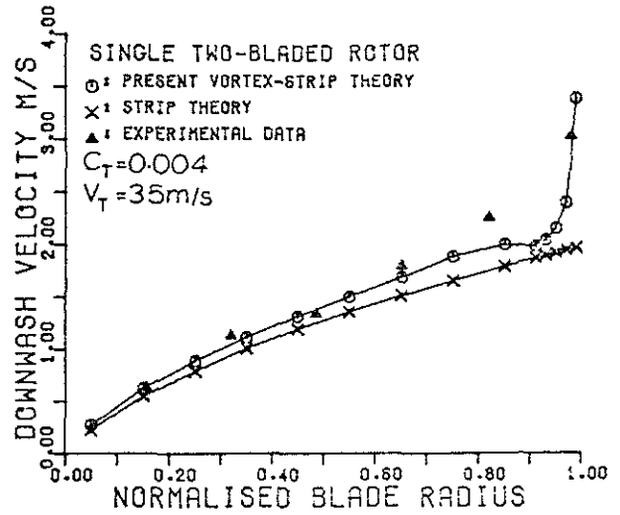
Fig.2 Comparison of Strip and Vortex-Strip Theory
