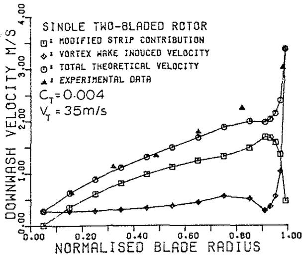
Fig.1 Component Downwash Velocity Distributions
