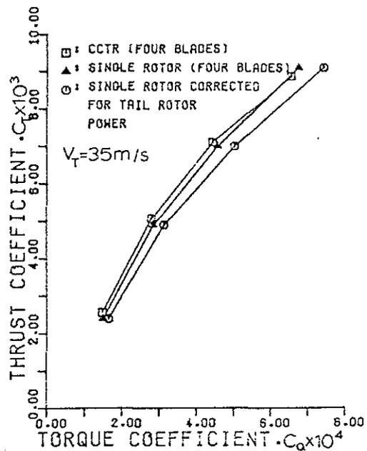
Fig. 6 Comparison of Performance Between an Equivalent Single Rotor and a CCTR
