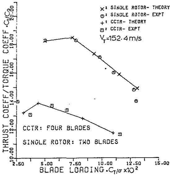
Fig. 5 Performance Curves for a Full-Scale CCTR
