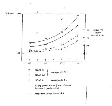
Figure 7 - Fatigue Life Usage on DRA Research Puma due to Longitudinal Cyclic Frequency Sweeps
