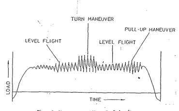
Figure 2 - Manoeuvre and Mean Cyclic Loads
