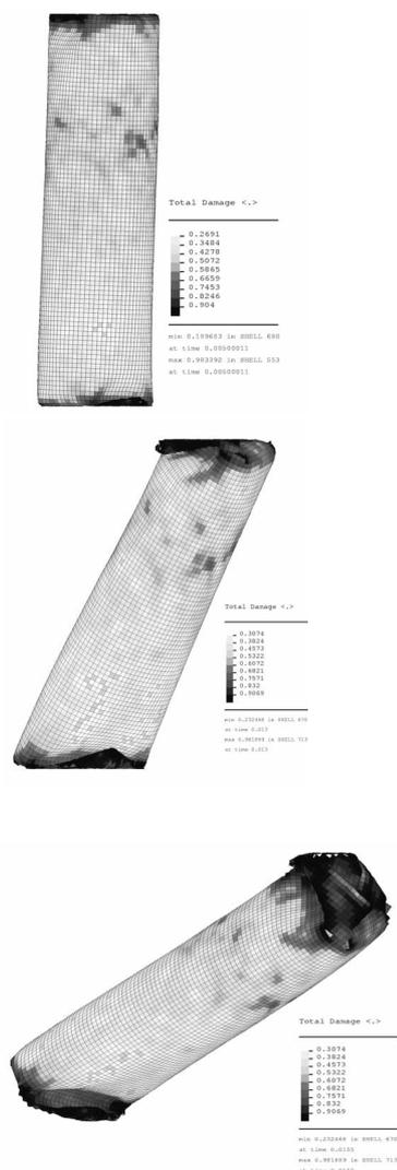
Fig 6. Sequence of the cylinder [-45°/45°]<sub>s</sub> numerical deformations
