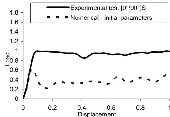
Fig 4. Normalized load-displacement curves of the cylinder typology with stacking sequence of  $[0^\circ/90^\circ]_s$
