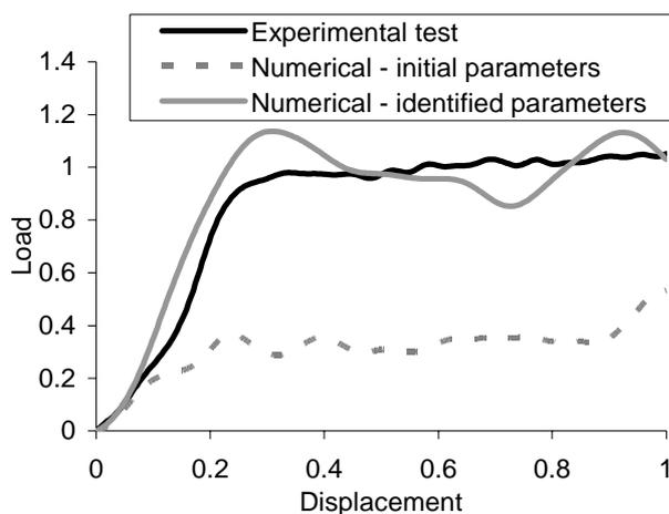
Fig 11. Comparison between the normalized load-displacement curves of the conical absorption structure
