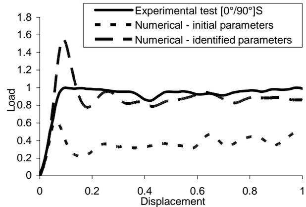
Fig 9. Comparison between the normalized load-displacement curves of the cylinders with stacking sequence  $[0^\circ/90^\circ]_S$
