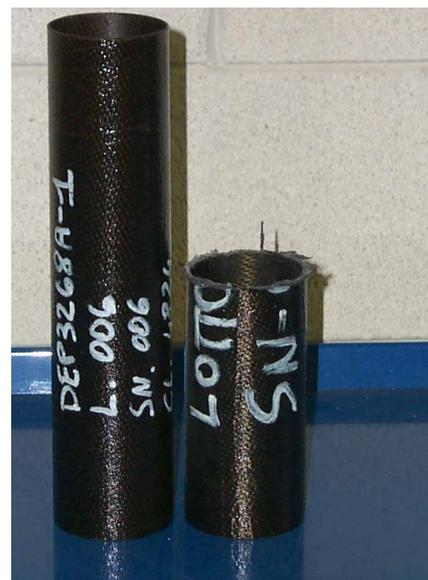
Fig 3. Tested specimen before and after vertical crashes
