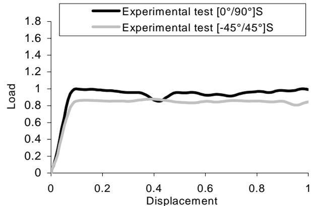
Fig 2. Normalized load-displacement curves of the cylinder typologies with  $[0^\circ/90^\circ]_S$  and  $[-45^\circ/45^\circ]_S$  stacking sequences
