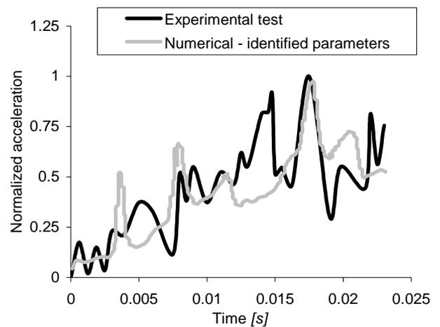
Fig 15. Numerical and experimental acceleration-time diagrams of the FSS
