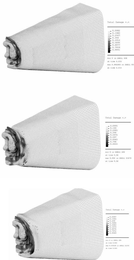
Fig 16. deformed shape evolution of the Frontal Sacrificial Structure
