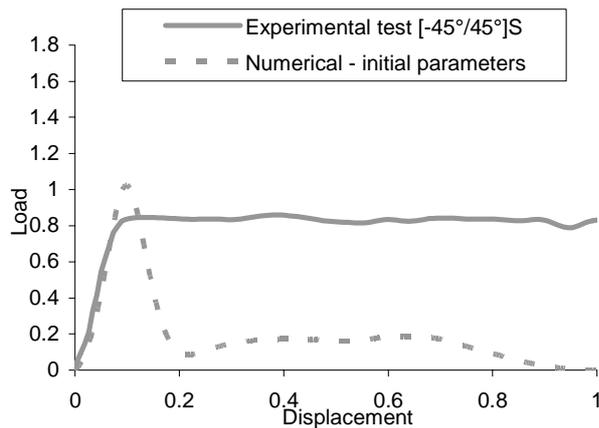
Fig 5. Normalized load-displacement curves of the cylinder typology with stacking sequence of [-45°/45°]<sub>s</sub>
