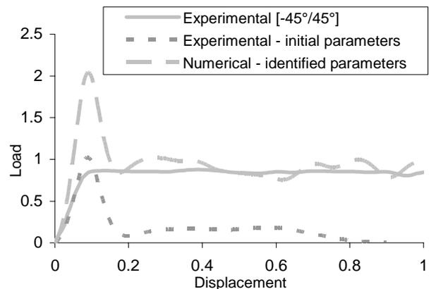
Fig 10. Comparison between the normalized load-displacement curves of the cylinders with stacking sequence  $[-45^\circ/45^\circ]_S$
