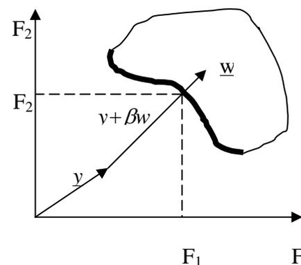
Fig 7. Goal-attainment method with two objective functions
