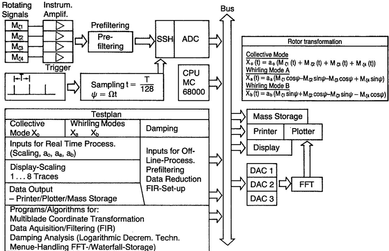
Fig. 18 Test Procedure for Investigation of Rotor Modes
