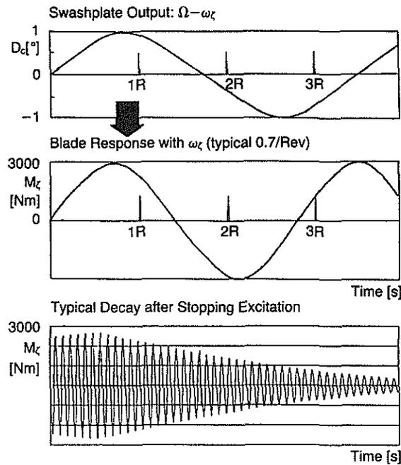
Fig. 14 Periodical Monocyclic Input and Decay of Inplane Bending Moment after Excitation.
