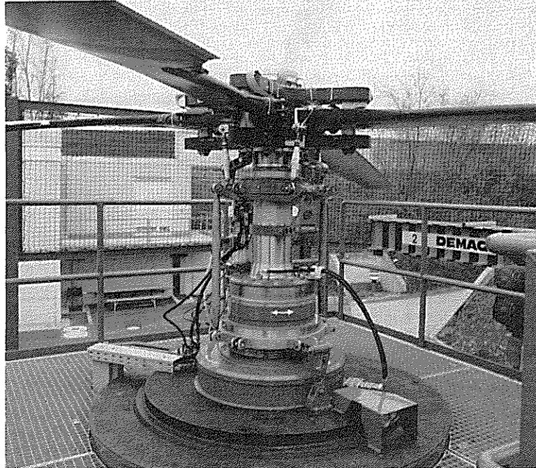
Fig. 3 MBB-RPS60, Blade Control System
