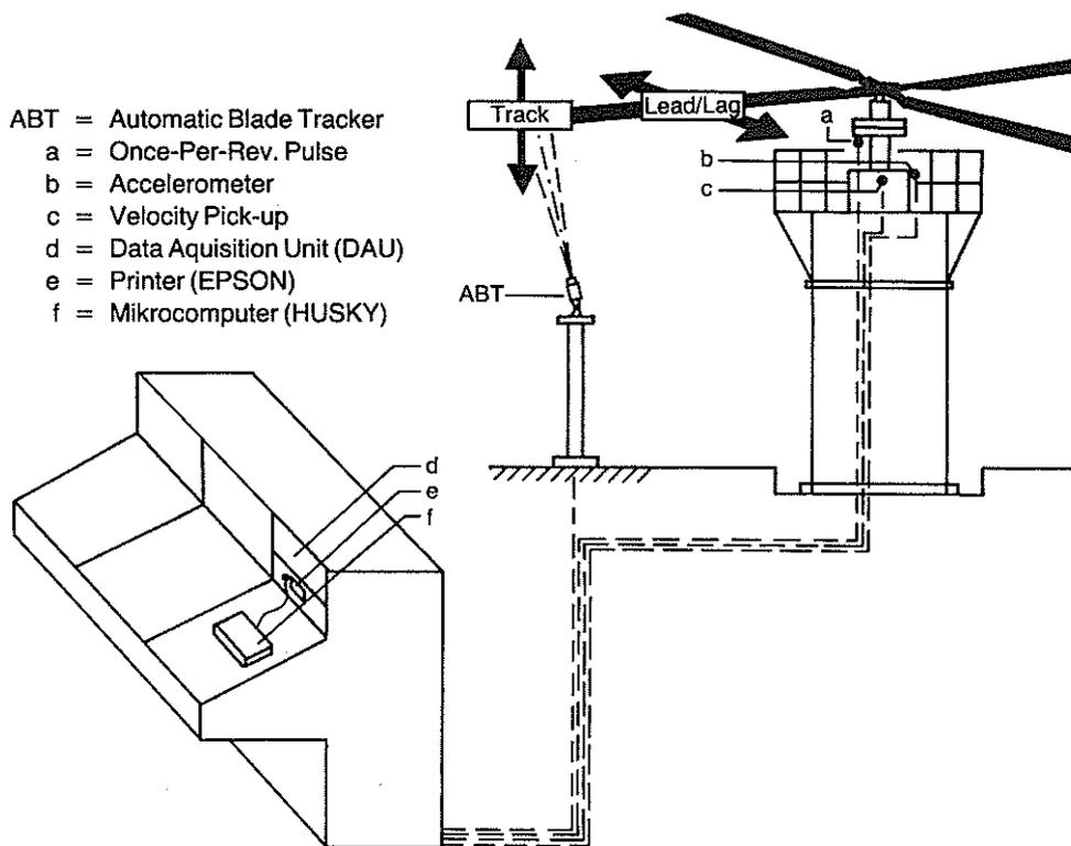
Fig. 23 Rotor Analysis Development System (RADS, Stewart Hughes)
