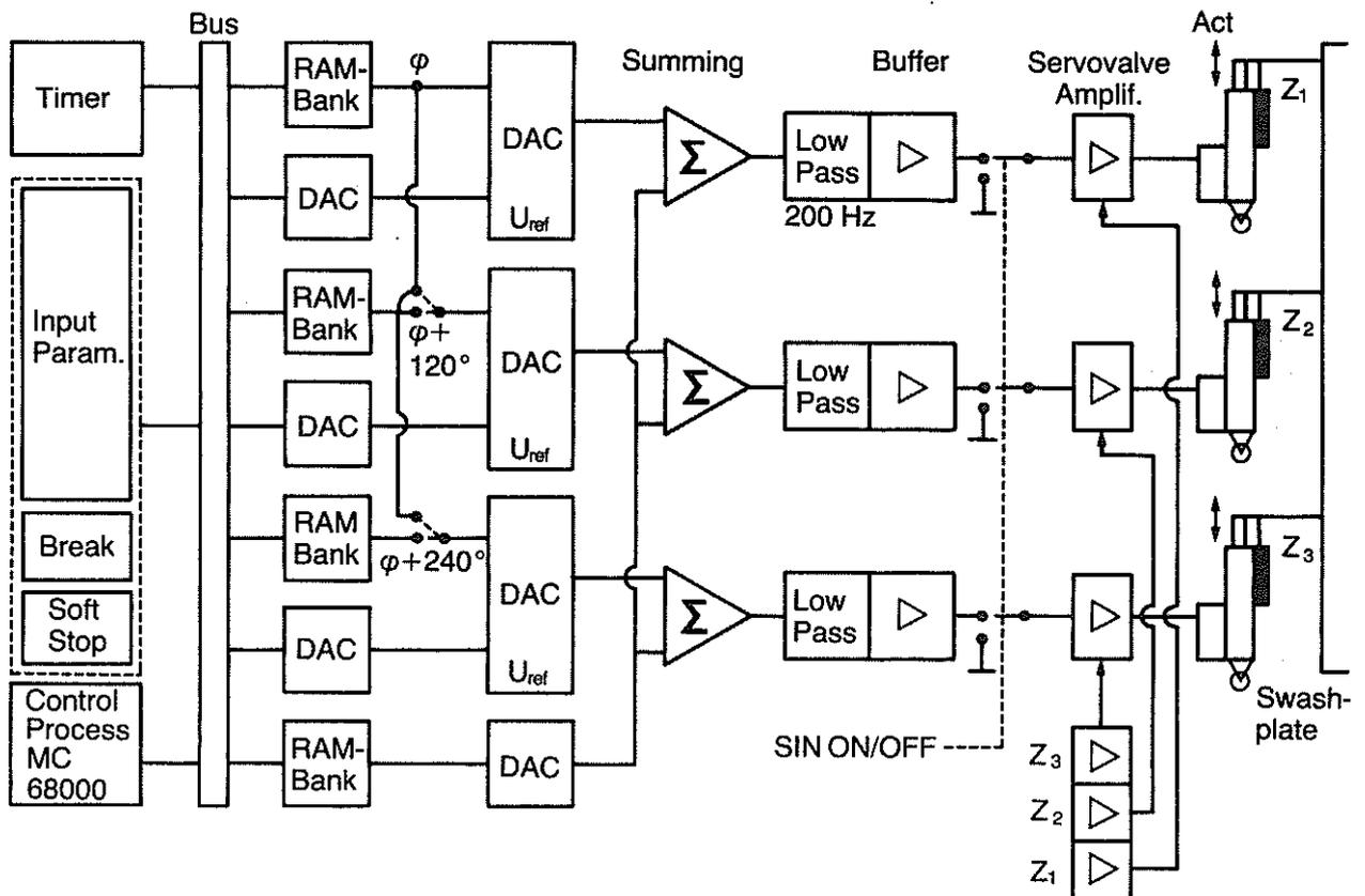
Fig. 17 Actuator Control Processing System
