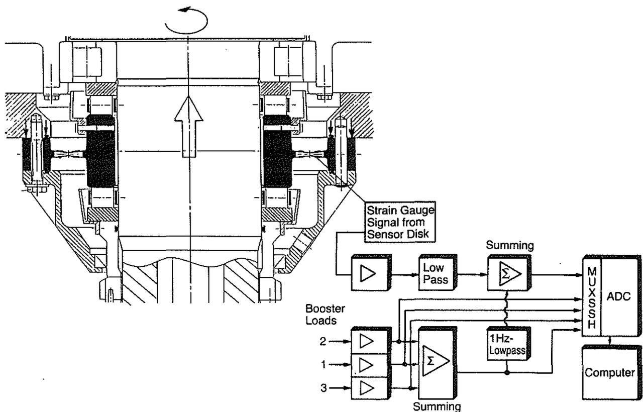
Fig. 20 Rotor Thrust Measuring, Data Acquisition
