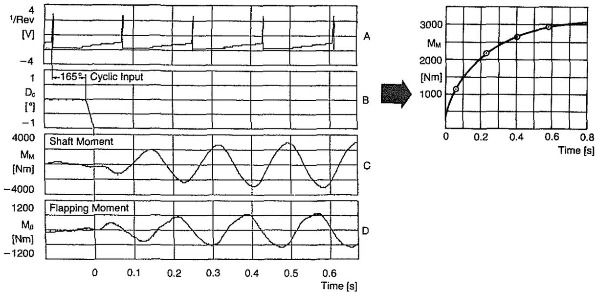
Fig. 13 Increase of Control Moment Owing to Cyclic Control Input of  $D_c = 1^\circ$
