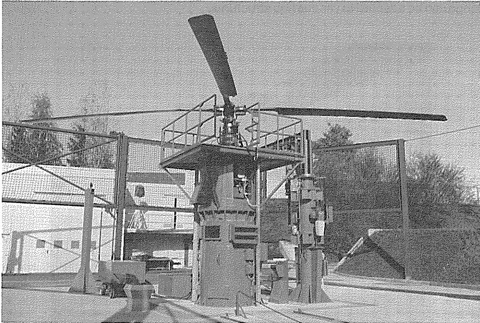
Fig. 1 MBB-RPS60, Rotary Test Rig
