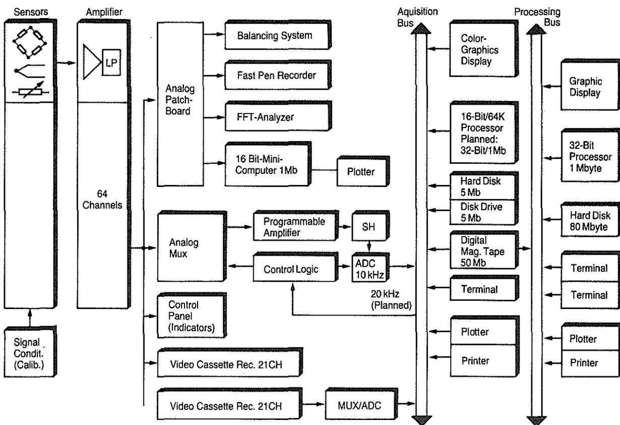
Fig. 22 Block Diagram of Data Acquisition and Processing System
