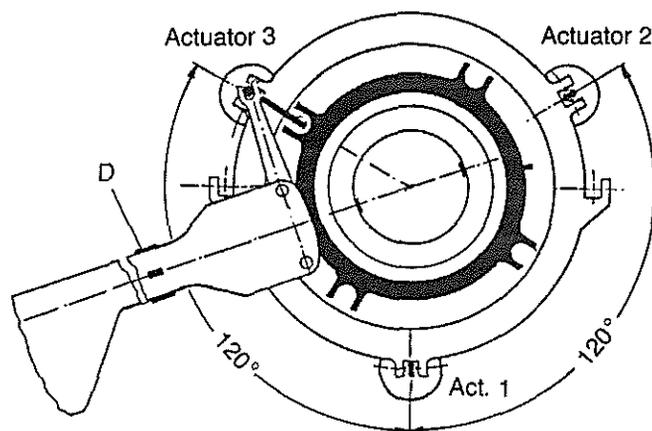
Fig. 15  $3 \times 120^\circ$ -Swashplate Support
