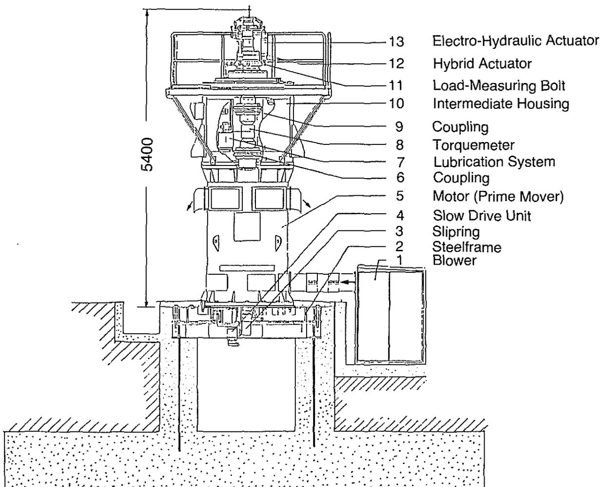
Fig. 5 60 KN-Rotary Test Rig
