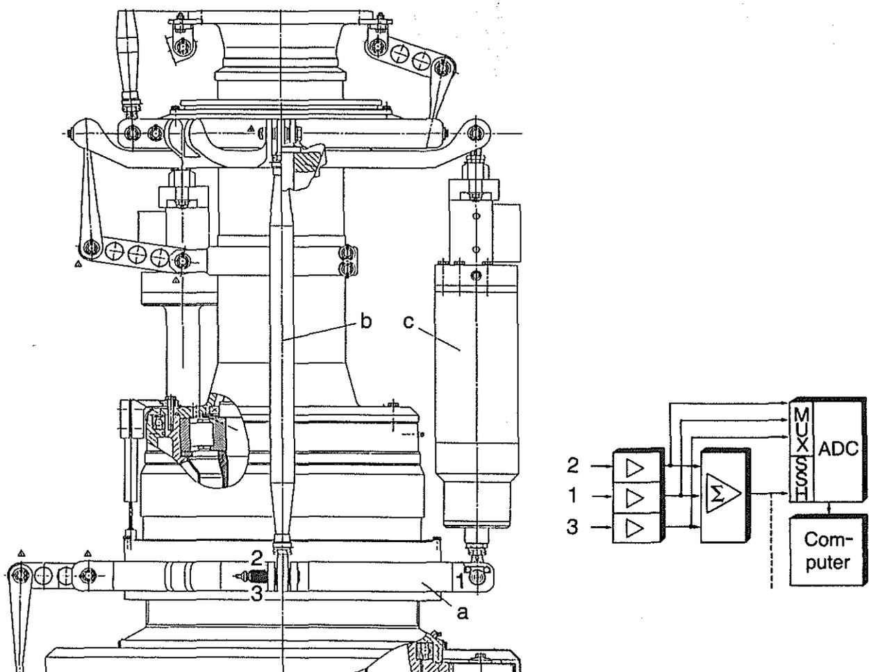
Fig. 19 Booster Load Measuring
