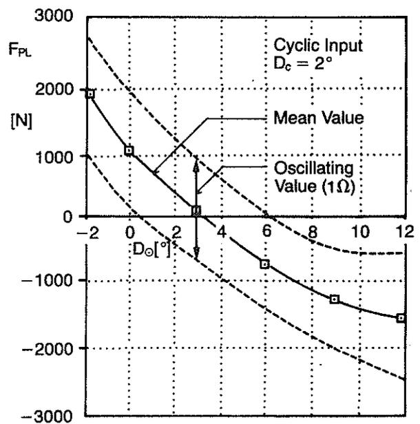
Fig. 11 Effect of Steady-State Cyclic Input on Pitch Link Load
