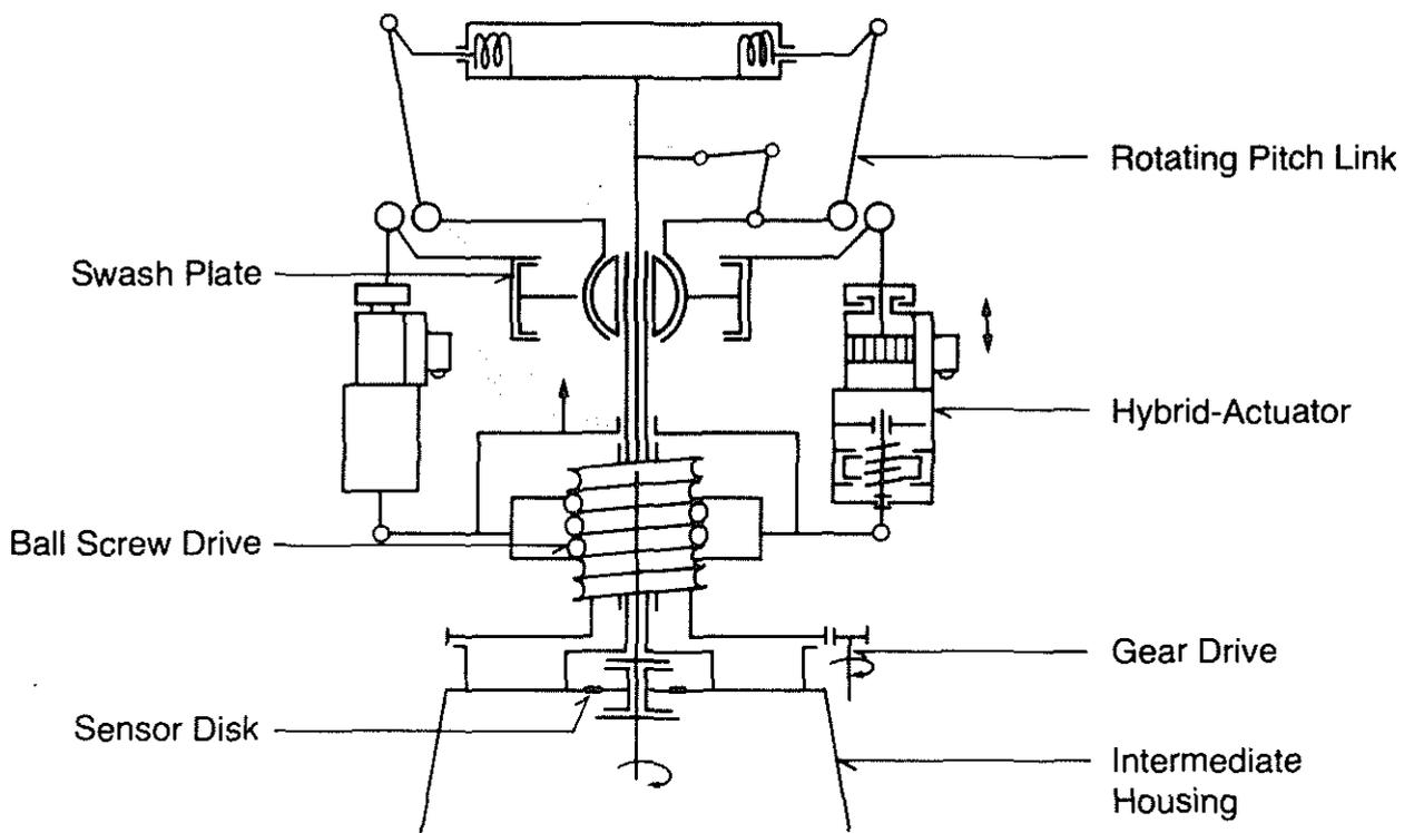
Fig. 7 Collective Pitch Control, Schematic
