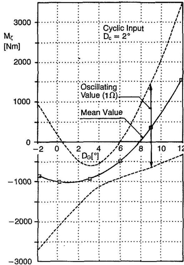
Fig. 12 Response of Inplane Bending Moment after a Steady State Cyclic Input of  $D_c = 2^\circ$
