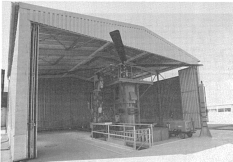
Fig. 2 MBB-RPS60, Rotary Test Rig with Dolly and Removable Hangar
