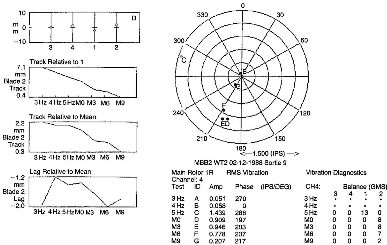
Fig. 24 Track/Lag- and Balancing Polar Plot during Run-up and Steady-State at Different Collective Pitch
