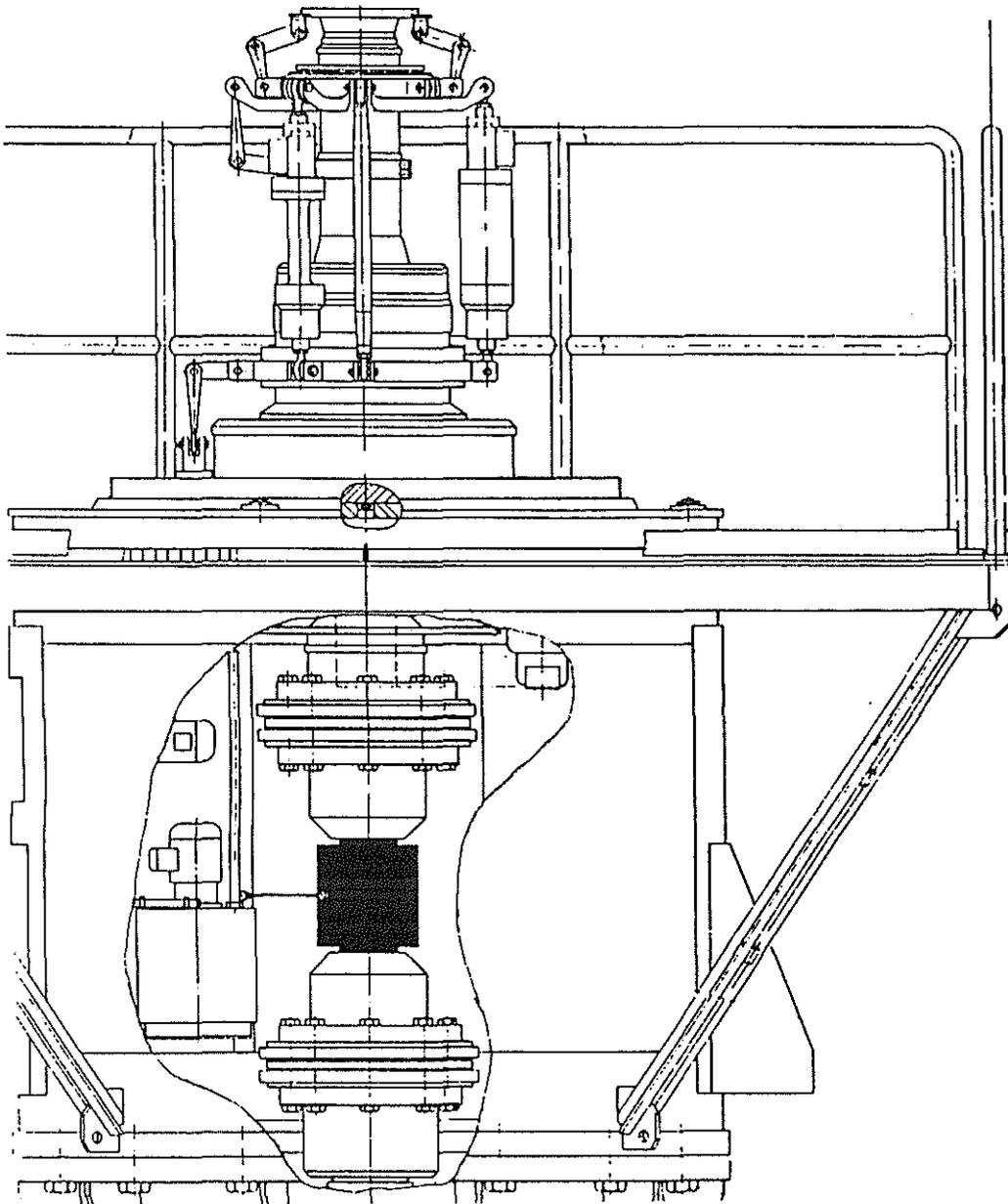
Fig. 21 Torque Measuring System
