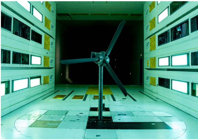
Figure 1: ATTILA testbed in the DNW Large Low-speed Facility (LLF) 6 m \times 6 m wind tunnel test section.
