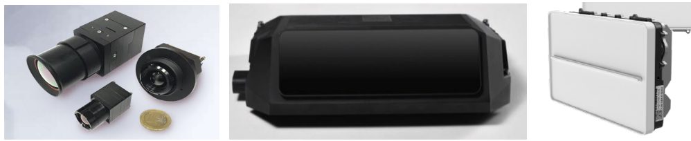
Fig. 1. Example of IR cameras, Lidar and Radar for SAA
