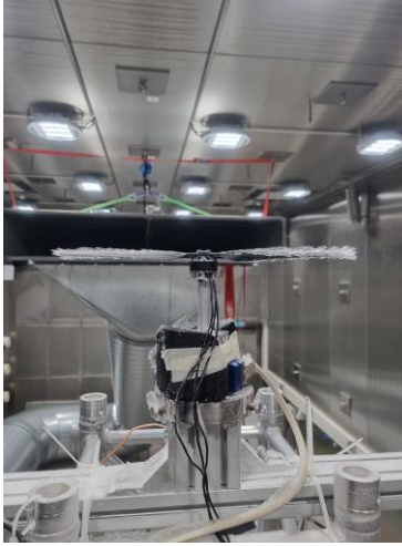
Figure 2. Single-rotor test setup
