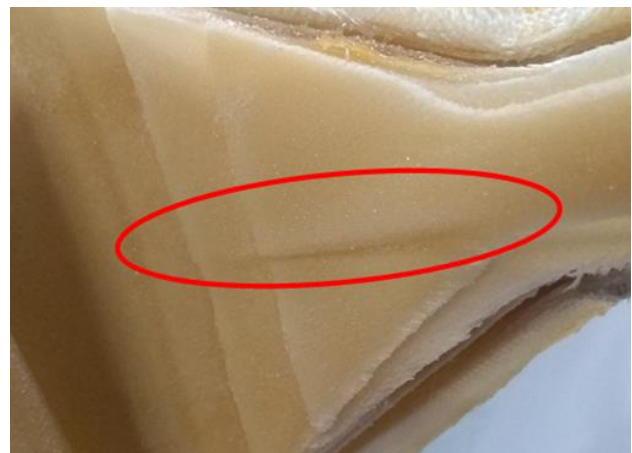
Figure 1: Ripple ("wrinkle") defect
