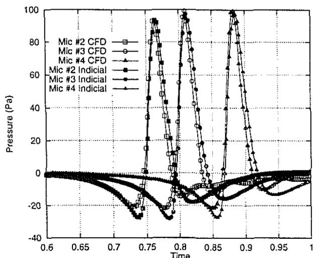
Figure 3: Acoustic signature for BVI at 180° using indicial method and CFD method to calculate unsteady aerodynamic loads at  $M_{tip} = 0.71$  and  $\mu = 0.2$ .
