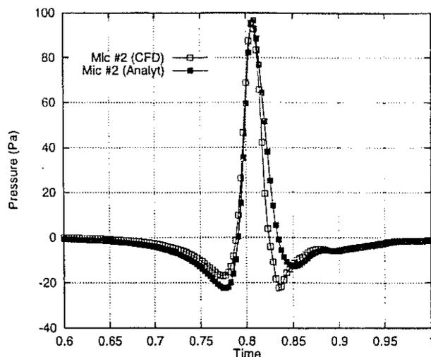
Figure 2: Comparison of acoustic signature for analytical chordwise pressure distribution and the CFD predicted chordwise pressure distribution for BVI at  $M_{tip} = 0.71$  and  $\mu = 0.2$ .
