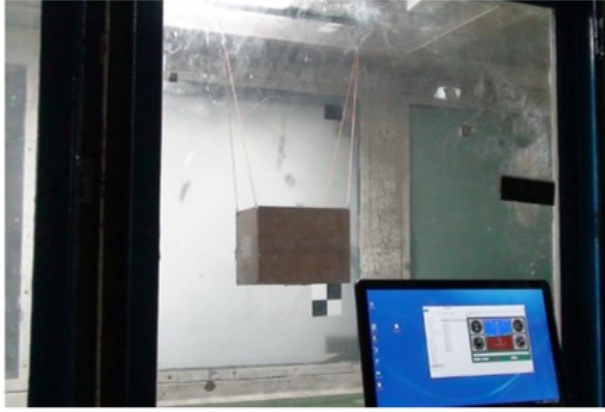
Figure 1: Wind tunnel test set-up (first phase)
