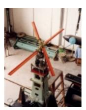
Fig. 1 Scissors rotor on the 2-m rotor rig
