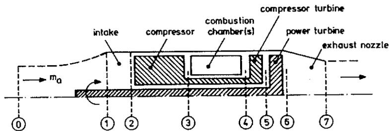
Fig. 1. Shaft-power turbo engine with free turbine.
