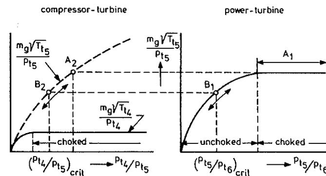
Fig. 4. Matching of the two turbines.
