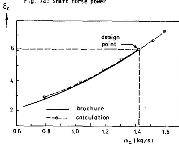
Fig. 7b: Compressor pressure ratio
