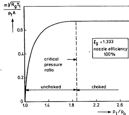
Fig. 3. Characteristic curve for exhaust nozzle.
