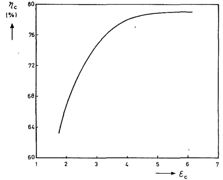
Fig. 6. Compressor efficiency.
