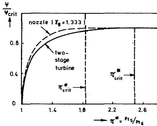
Fig. 5. Turbine mass flow according to Linnecken ( $\pi_{crit}^* = 2.5$ ).
