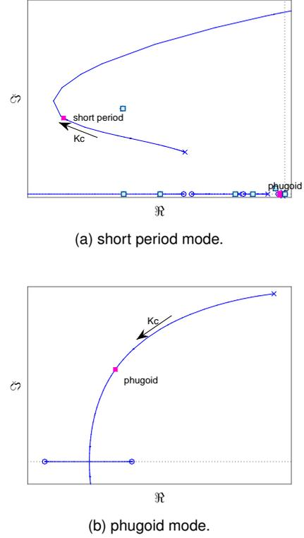
Figure 9: C\* root locus (varying loop gain  $K_{cp}$ ).
