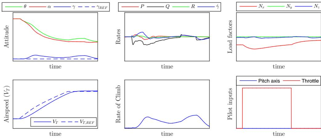
Figure 12: Throttle response in airplane mode.
