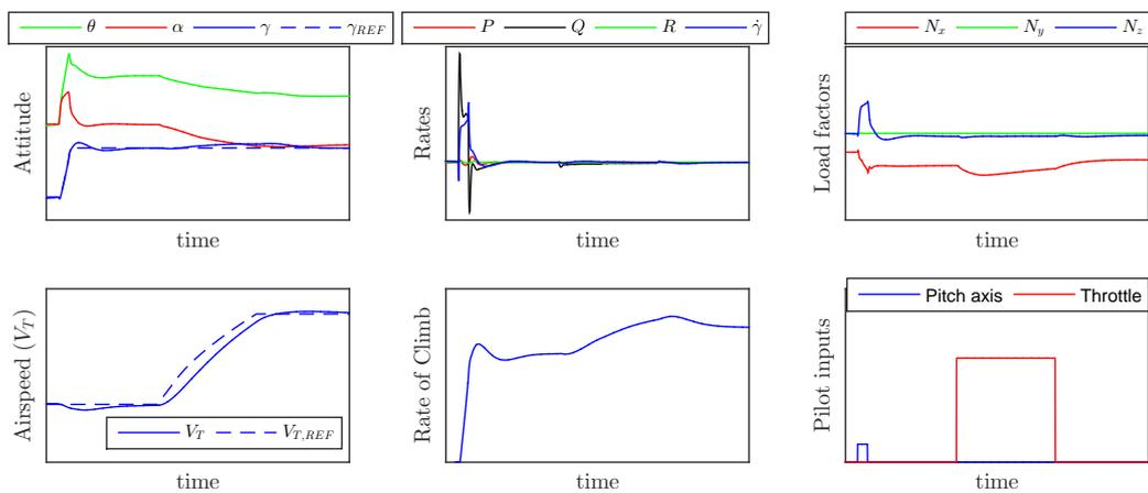
Figure 13: Pitch and throttle response in airplane mode.
