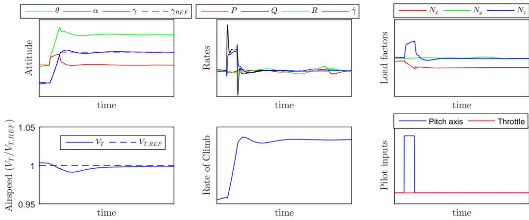
Figure 11: Pitch response in airplane mode.
