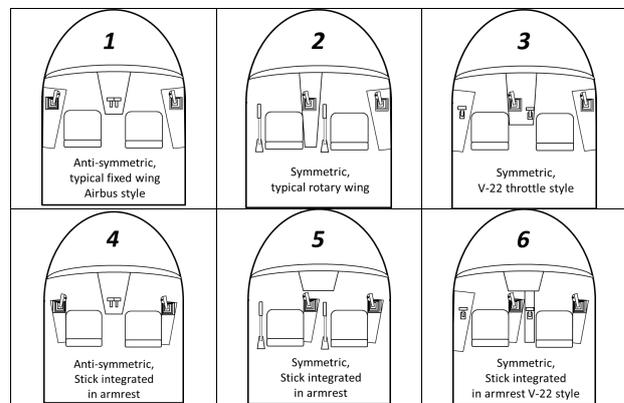
Figure 1: Tiltrotor cockpit layout options.
