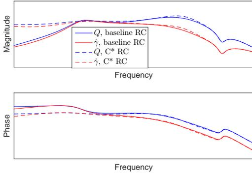
Figure 8: C\* frequency response, from  $\delta_{LON}(j\omega)$  to  $Q(j\omega)$  and  $\dot{\Gamma}(j\omega)$ , compared to baseline rate command system.
