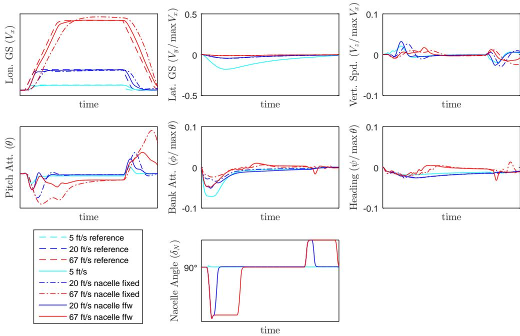
Figure 3: TRC longitudinal responses, commanded vs. fixed nacelle angle.
