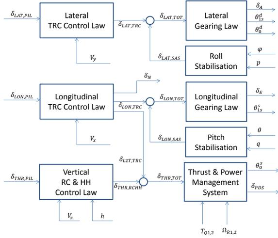
Figure 2: Longitudinal/Lateral TRC and Vertical RCHH control concept applied to Tiltrotor.
