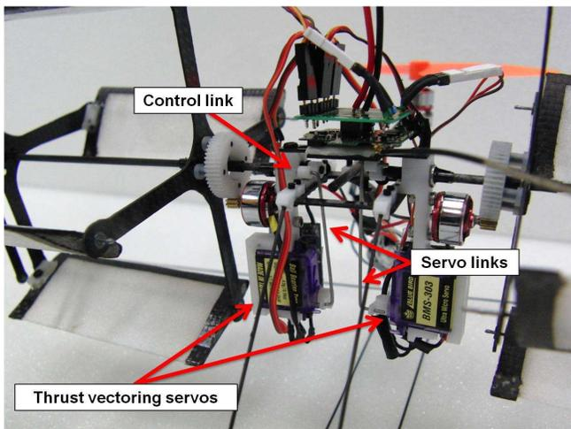
Figure 9: Thrust vectoring mechanism.
