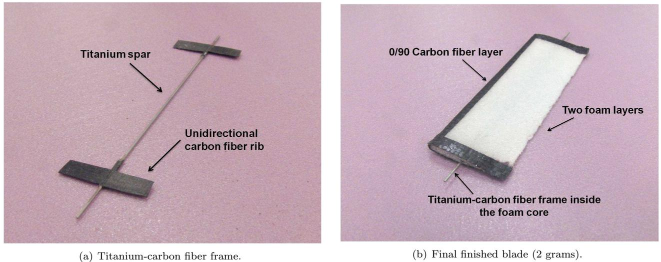
Figure 7: Cyclorotor blade design.
