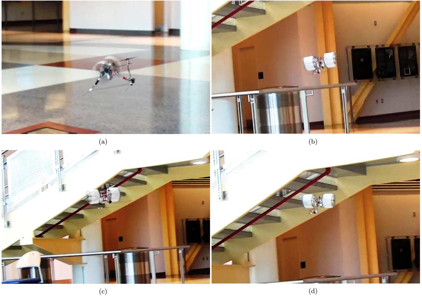
Figure 17: **Autonomous stable hover of the 110 gram twin-cyclocopter.**
