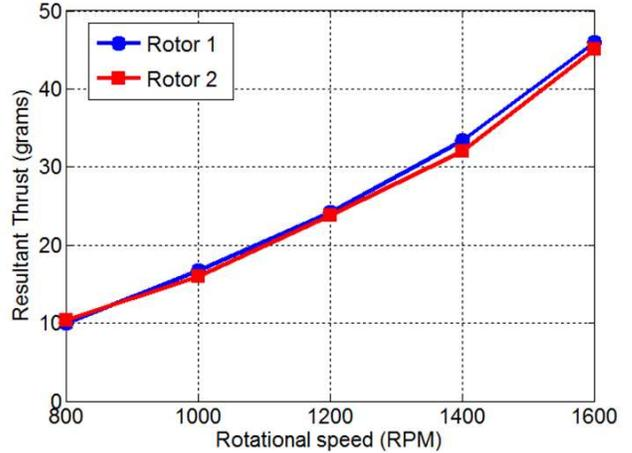
Figure 10: Thrust vs. rotational speed of the two cyclorotors.
