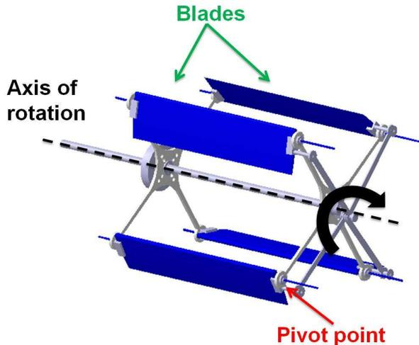
Figure 1: Cycloidal rotor.
