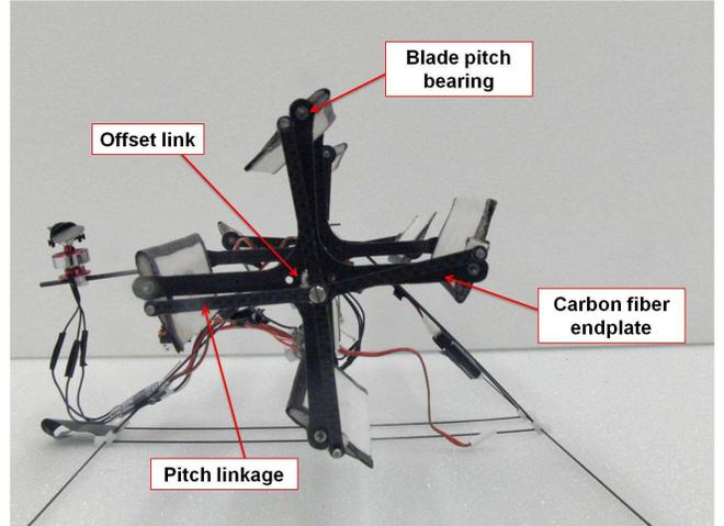
Figure 6: Four-bladed cyclorotor.
