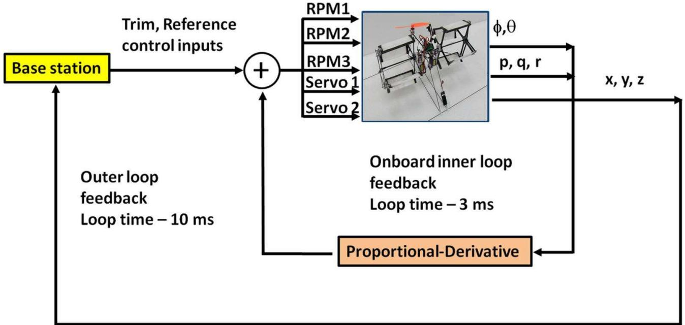
Figure 16: Schematic showing the inner-loop feedback control system implemented.
