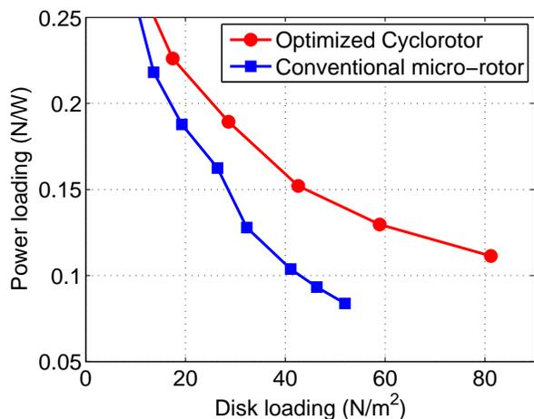
Figure 3: Power loading (thrust/power) vs. disk loading (conventional micro-rotors vs. optimized cyclorotor) [7].
