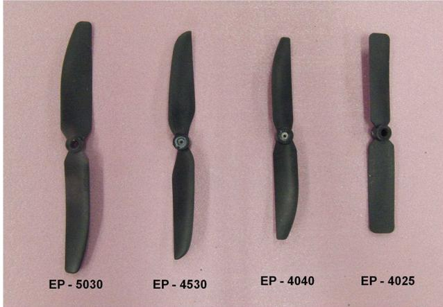
Figure 12: Variation of tail rotor propellers tested.
