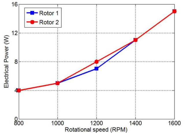
Figure 11: Power required vs. rotational speed of the two cyclorotors.
