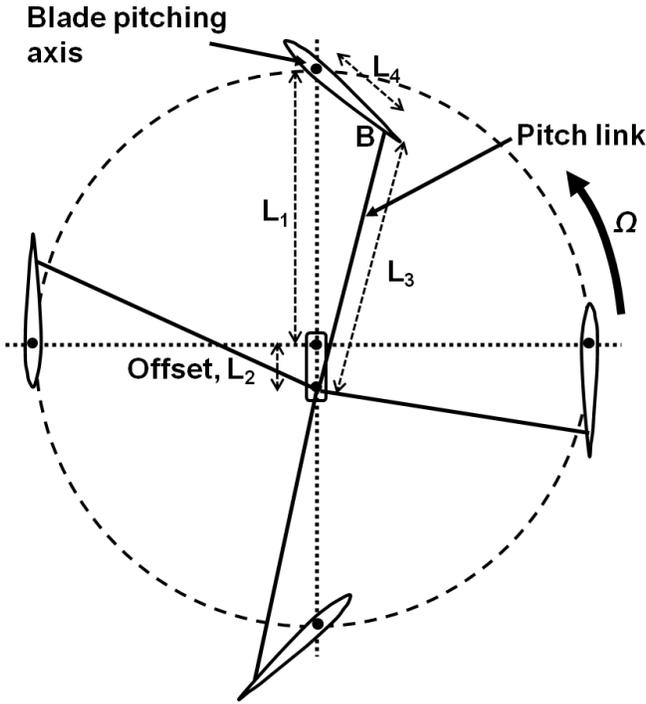
Figure 8: Schematic of the blade pitching mechanisms.
