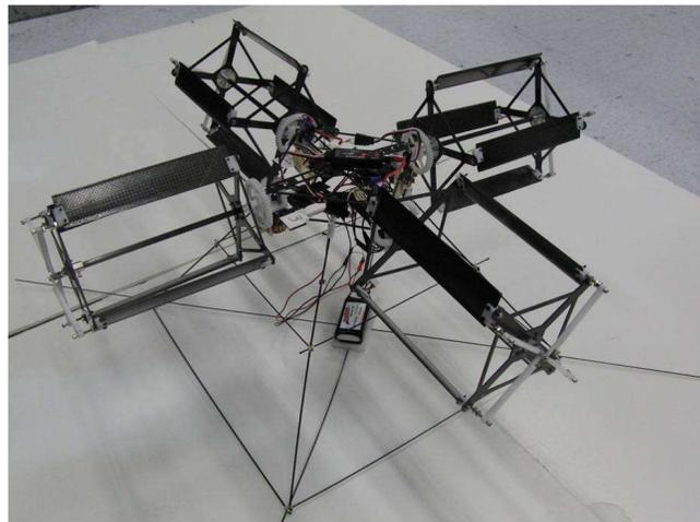
Figure 4: 800 grams quad-cyclocopter developed by the University of Maryland [13].
