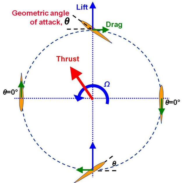
Figure 2: Blade pitching kinematics.
