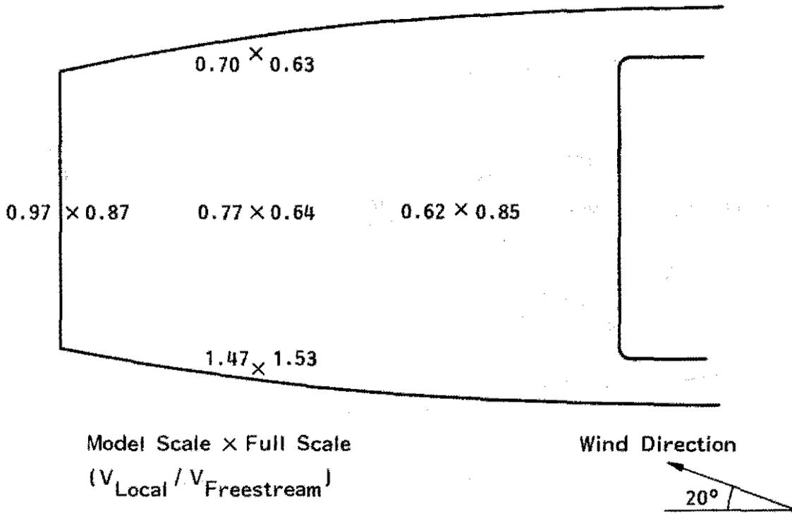
Figure 6 COMPARISON OF MODEL AND FULL SCALE VELOCITIES
