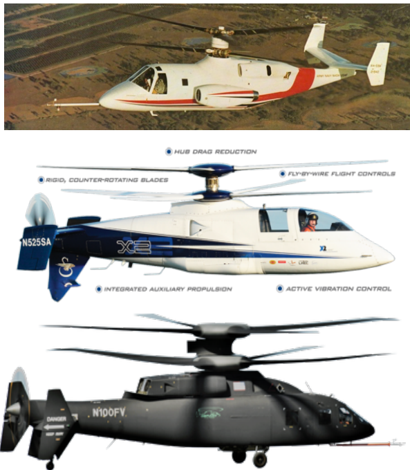
Figure 1. Evolution of Lift-Offset Coaxial Rotor Vehicles with Auxiliary Propulsion. From top to bottom: XH-59A, X2, S-97 (Ref. 11, Ref. 12).
