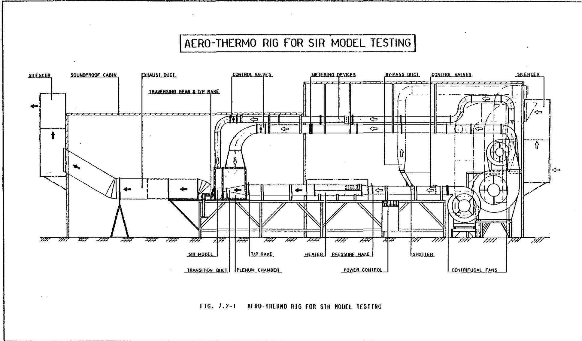
FIG. 7.2-1 AERO-THERMO RIG FOR SIR MODEL TESTING
