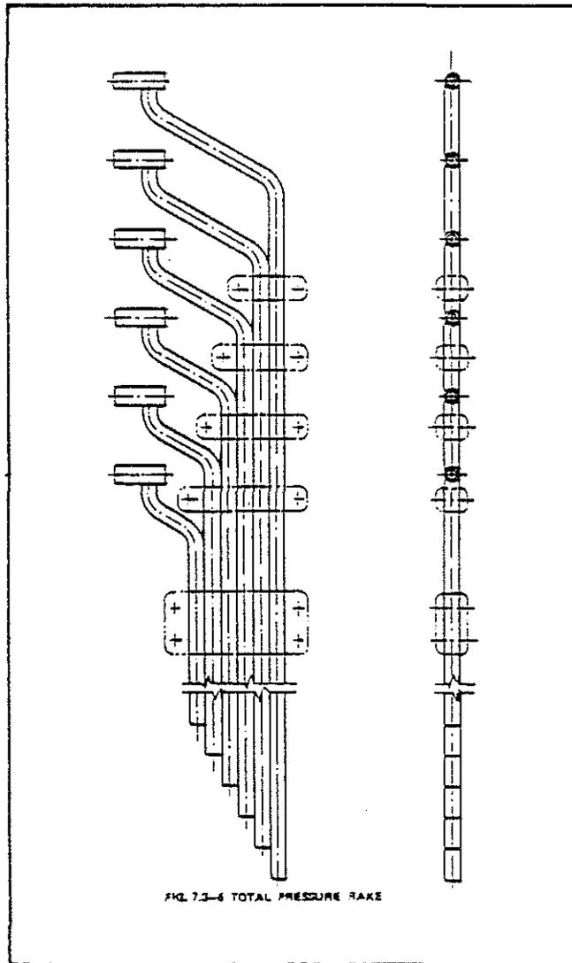
FIG. 7.3-6 TOTAL PRESSURE RAKE
